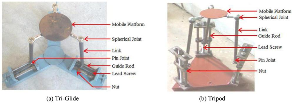
Fig. 3. prototype model of PMs
