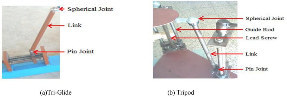
Fig. 2. one link arrangement of PMs
