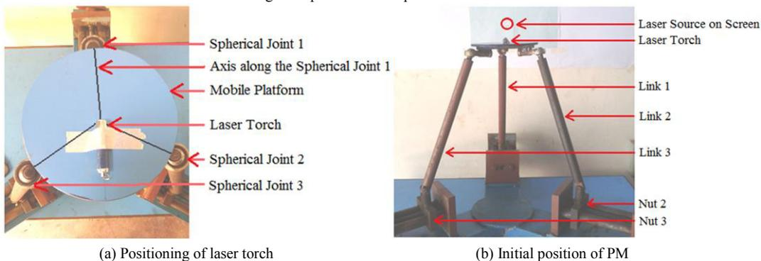
Fig. 6. PM with laser torch
