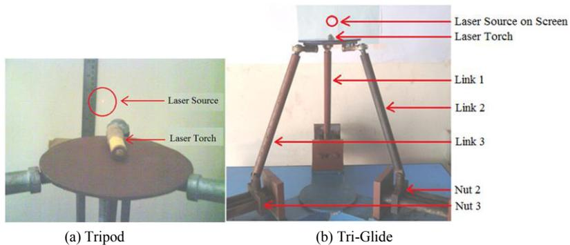
Fig. 5. experimental setup with laser torch
