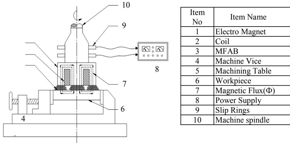
Fig 1. Schematic view of MFAAF Experimental Setup spindle assembly [20]
