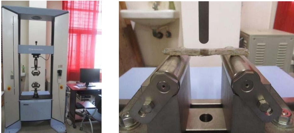
Figure 3. (a) Universal testing machine; (b) Flexural test setup (Courtesy : Strength of materials lab, VIT University, Chennai)
