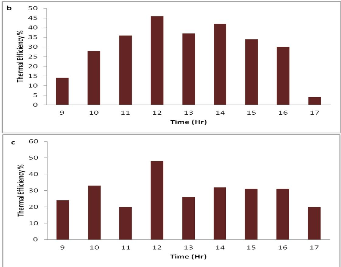
Fig. 2. (a) Thermal efficiency of SWH with clear glass and tilt angle of 15° (b) Thermal efficiency of SWH with clear glass and tilt angle of 20° (c) Thermal efficiency of SWH with clear glass and tilt angle of 25°
