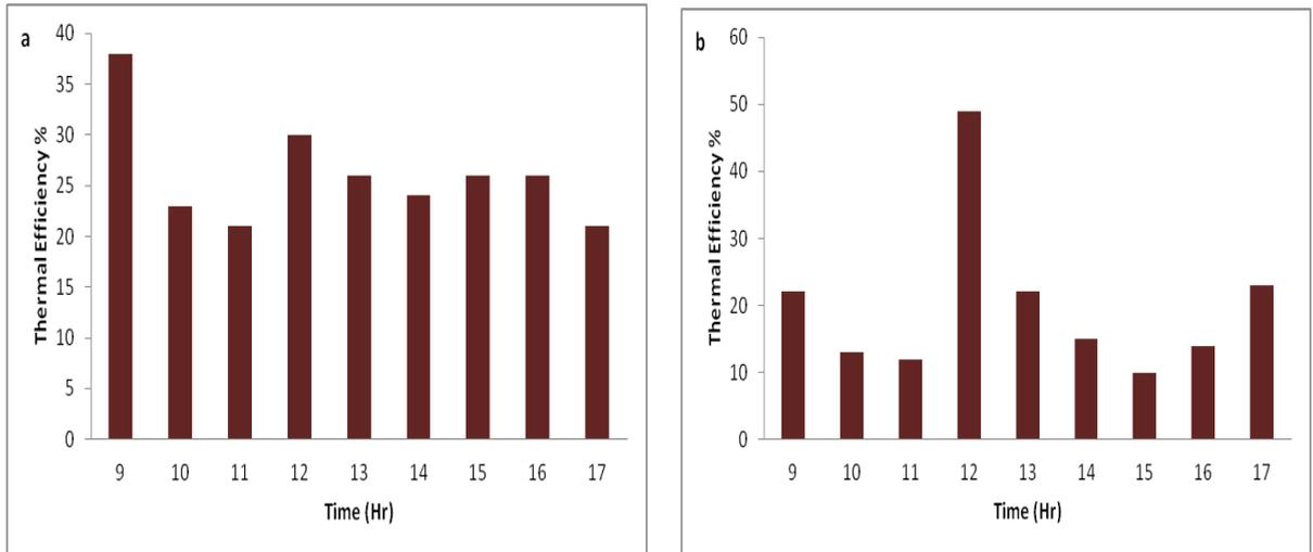
Fig. 3. (a) Thermal efficiency of SWH with clear glass and tilt angle of 25° (b) Thermal efficiency of SWH with partially dusty glass and tilt angle of 25°
