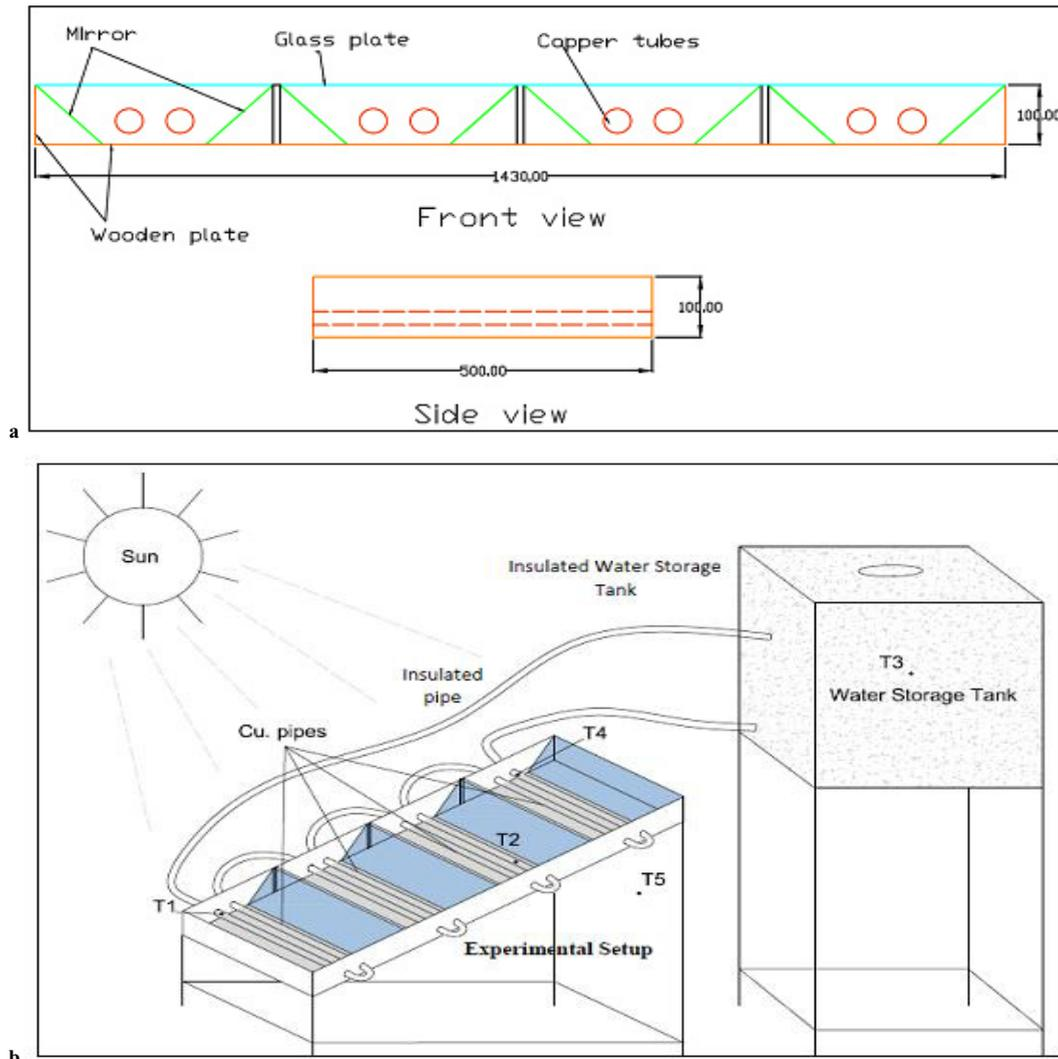
Fig. 1. (a) Elevation and side view of experimental set-up (b) Schematic diagram of experimental set-up
