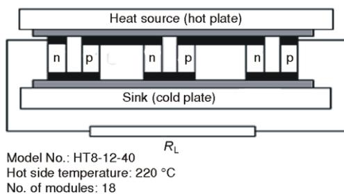
**Figure 1. TEM connected to the load**
