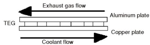
Figure 9. Schematic diagram of the TEM sandwiched between the hot plate and cold plate
