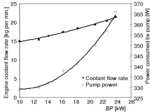
Figure 12. Variation of engine coolant flow rate with brake power
