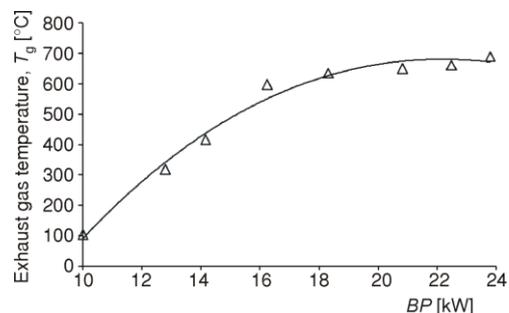
**Figure 16.** Variation of EGT with brake power
