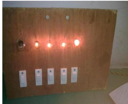
Figure 18. Electric bulb load panel
