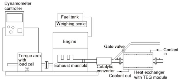
Figure 10. Schematic diagram of experimental set-up
