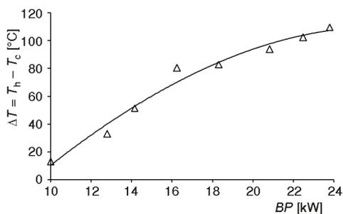
**Figure 17.** Variation of temperature difference with brake power
