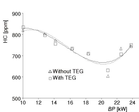
Figure 13. Variation of hydrocarbon emission with brake power
