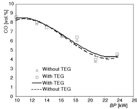
Figure 14. Variation of carbon monoxide emission with brake power
