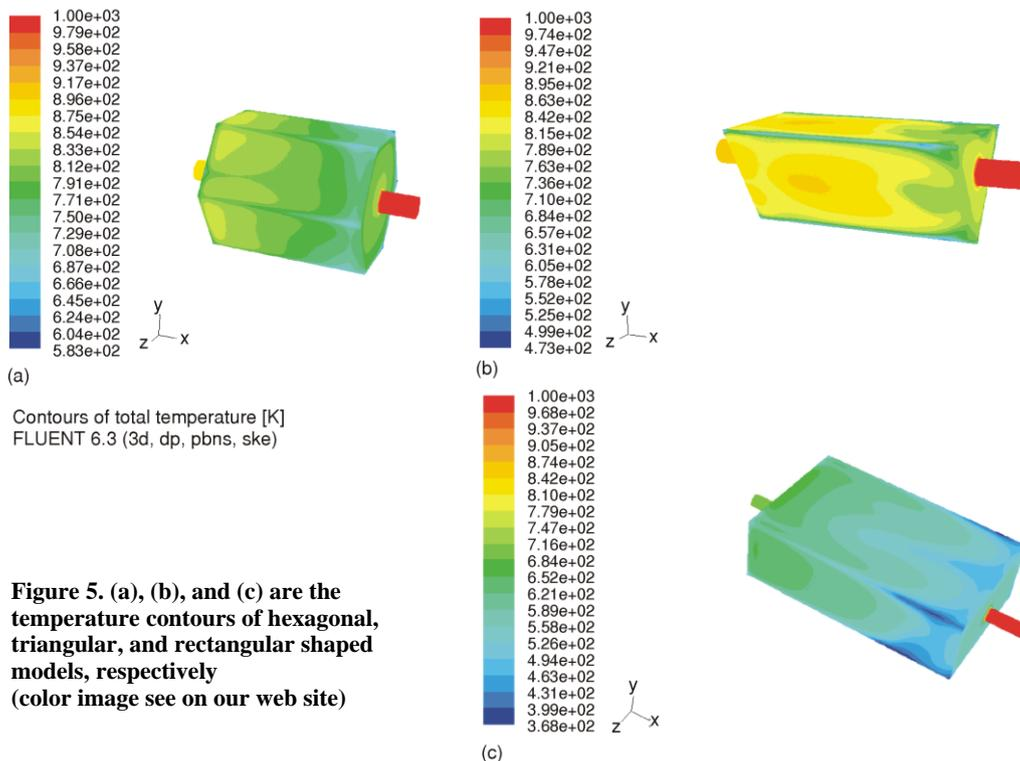
**Figure 5. (a), (b), and (c) are the temperature contours of hexagonal, triangular, and rectangular shaped models, respectively (color image see on our web site)**
