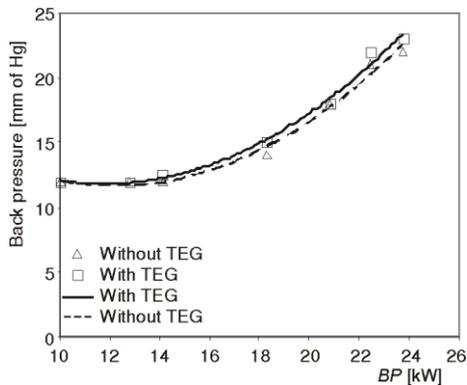
Figure 11. Variation of back pressure with brake power
