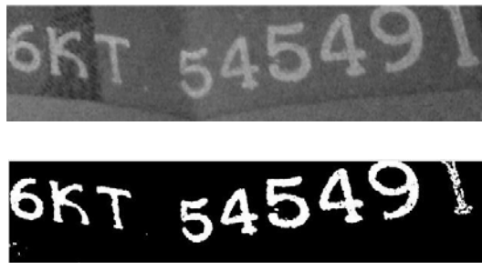
Figure 7. Edge based segmentation of serial number
