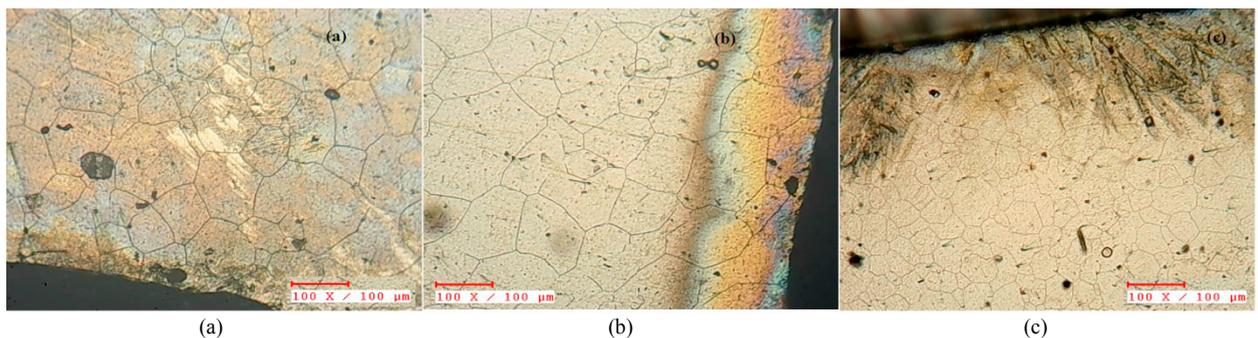
Fig. 8 Microstructure of heat affected zone of samples after SEDM in samples (a) 6 A (b) 12 A and (c) 20 A
