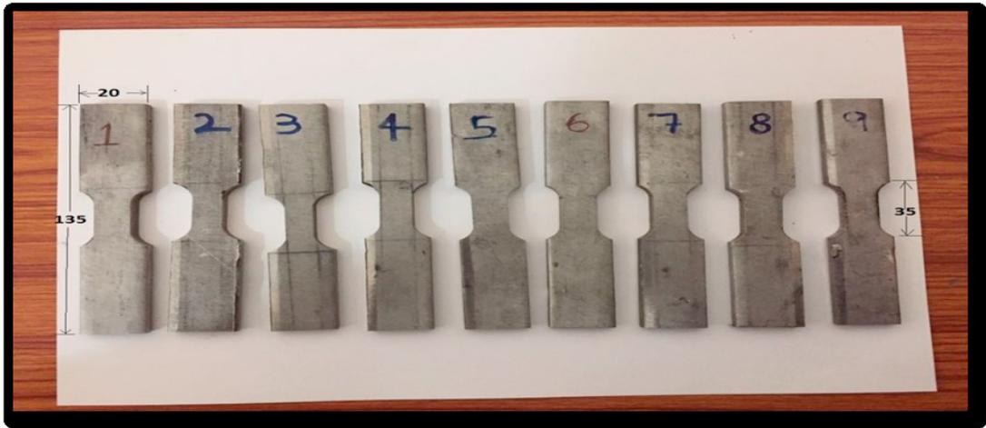
Fig. 5 ASTM E606 Fatigue Standard Samples.
