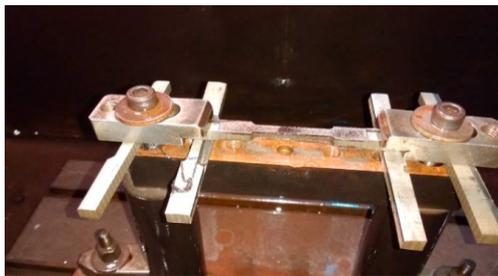
Fig. 3 Tool setup for the EDM process
