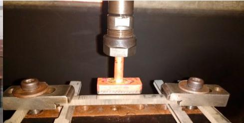
Fig. 2 Fatigue sample after EDM process
