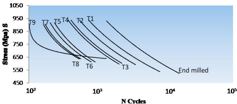
Fig. 9 S-N curve of SEDM samples compared with end milled
