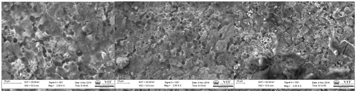
Fig. 6 SEM images of Inconel 718 after SEDM process.
