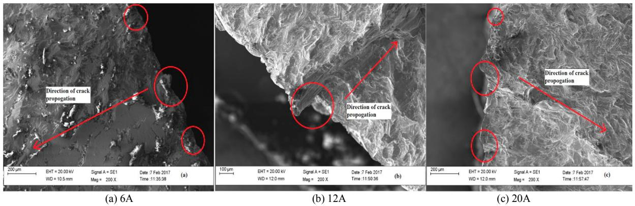
Fig. 7 Fractographs after fatigue test.
