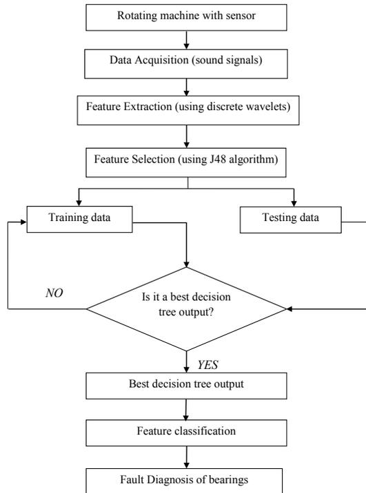
**Figure 1.** Floechart for roller bearing fault diagnosis.
