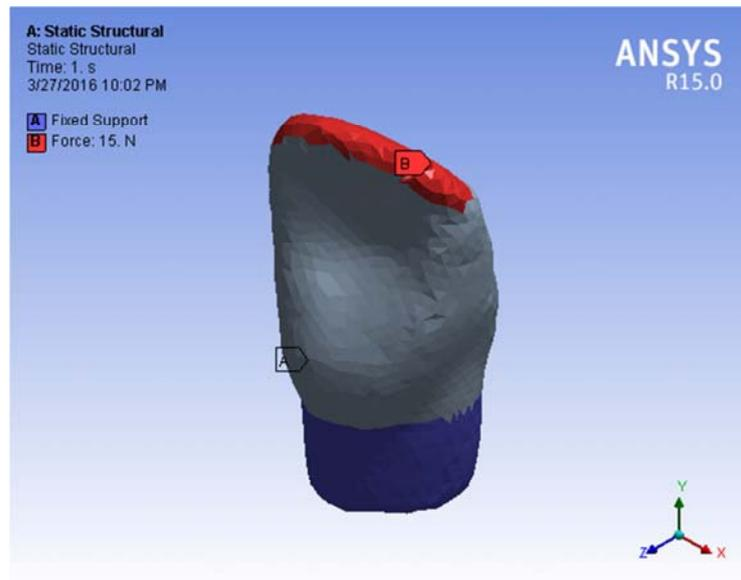
**Figure 5:** Application of horizontal force for case-2 with fixed base
