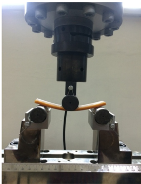
Figure 3. Sample undergoing flexural test.
