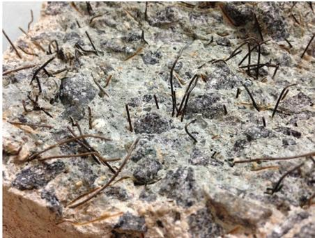
FIGURE 12: Fractured surface of geopolymer concrete showing fibre straining.
