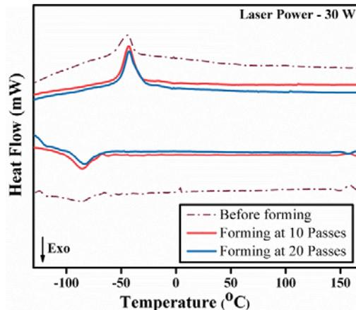
**Figure7-** DSC curves at 30 W power
