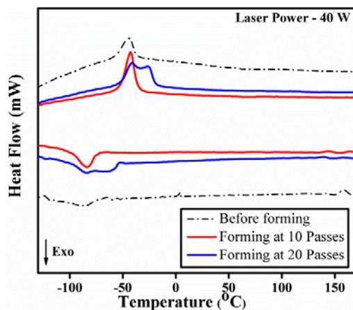
**Figure8-** DSC curves at 40 W power
