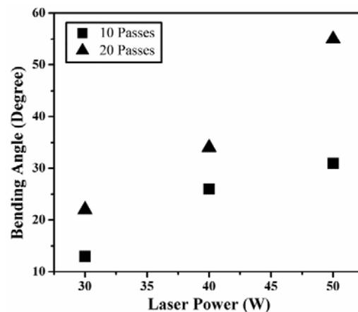
**Figure5-** Bending angle variation with number of passes
