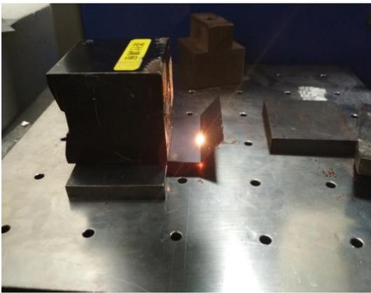
**Figure2** - Irradiation of laser on the Ni-Ti sheet.
