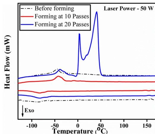
**Figure9-** DSC curves at 50 W power
