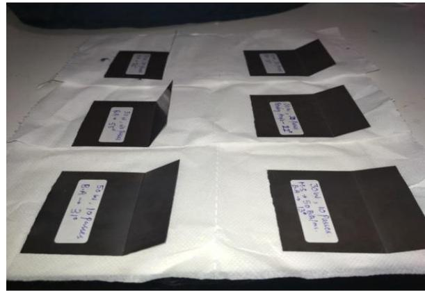
**Figure3** – Bended Ni-Ti samples after laser irradiation
