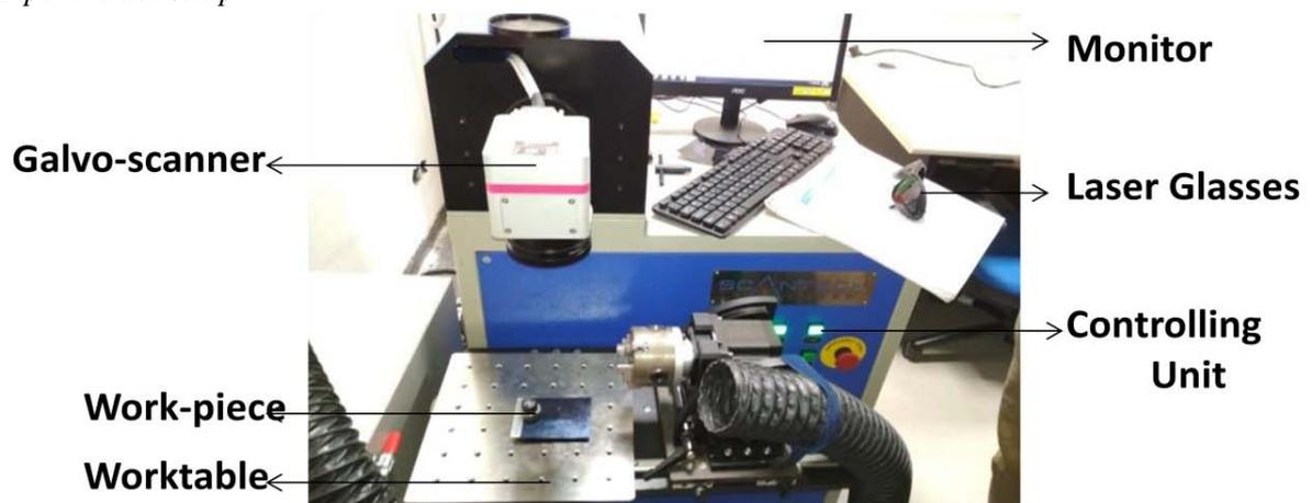
**Figure1** – Experimental setup used for laser forming
