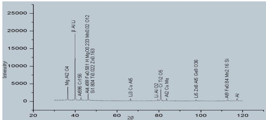
Fig. 6. X-Ray Diffraction results showing the formation of various phases at the stirred zone.
