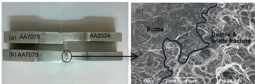
Fig. 5. Tensile studies on dissimilar weldments (a) before fracture (b) after fracture (c) SEM Fractograph.
