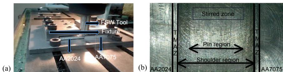
Fig. 1. Illustration of (a) FSW Process carried using conventional milling machine with the aid of specially designed fixture (b) Macrograph of the welded sample.
