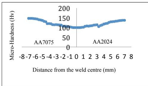
Fig. 4. Micro-hardness profile of the weldment
