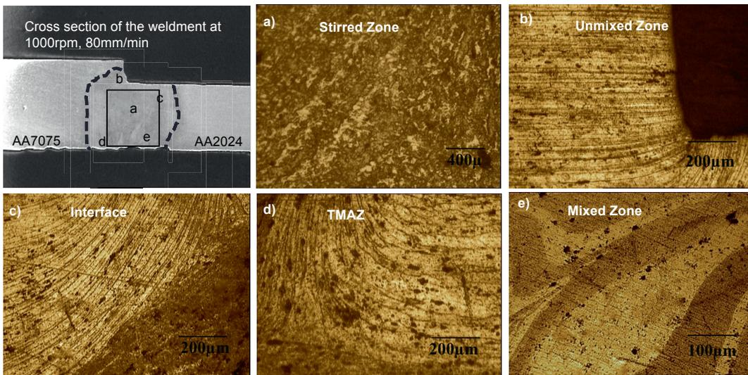
Fig. 2. Microstructure of (a) Stirred Zone (b) Unmixed region showing the thickness variation (c) Interface (d) TMAZ (e) Mixed flow region
