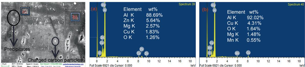
Fig. 3. SEM image of the stirred zone, and the corresponding EDAX analysis at (a) TMAZ and (b) nugget zone.
