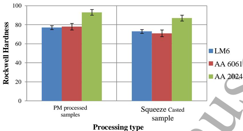
Figure 5: Comparison of Rockwell hardness of composites with 6 wt%  $Al_2O_3$
