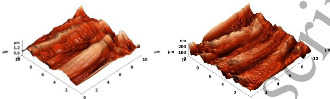
Figure 16: AFM Image of the AA 2024 P/M Pin wear track and Counter disc part wear track
