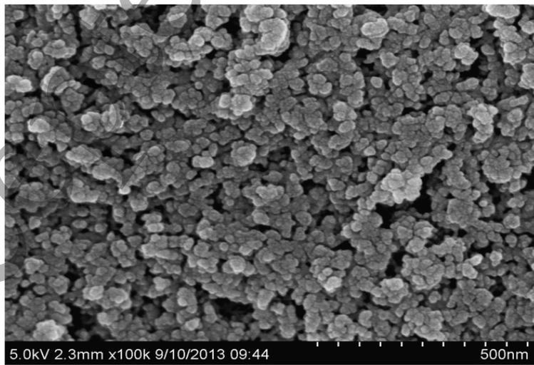
Fig 3: SEM Morphology of "as procured" Nano alumina
