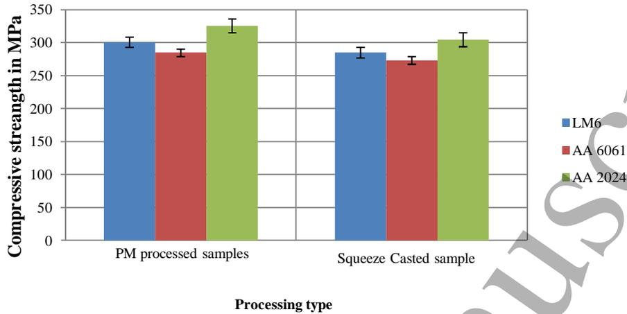
Figure 6: Comparison of compressive strength between composites
