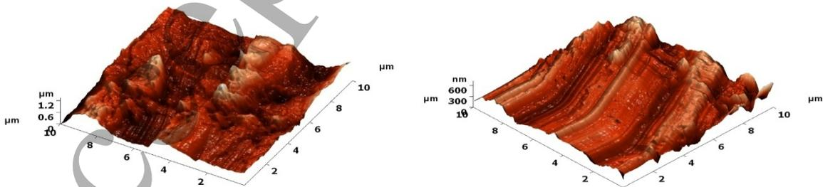
Figure 15: AFM Image of the AA 2024 P/M Pin wear track and Counter disc part wear track
