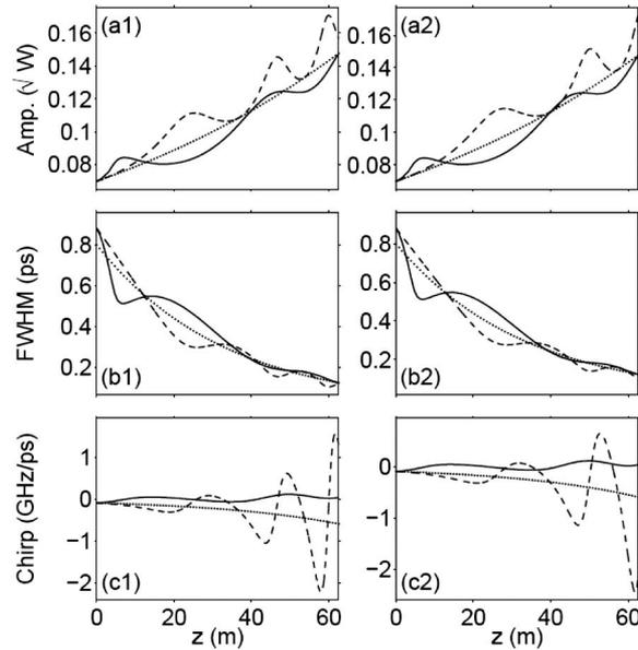
Fig. 16. Amplitude, pulsewidth, and chirp evolutions over  $8L_D$  distance propagation in CPCF. In Figs. (a1), (b1), and (c1) and (a2), (b2), and (c2), the dashed lines represent the results of LVM and CVM, respectively. The solid and dotted lines correspond to full numerical and analytical results, respectively.
