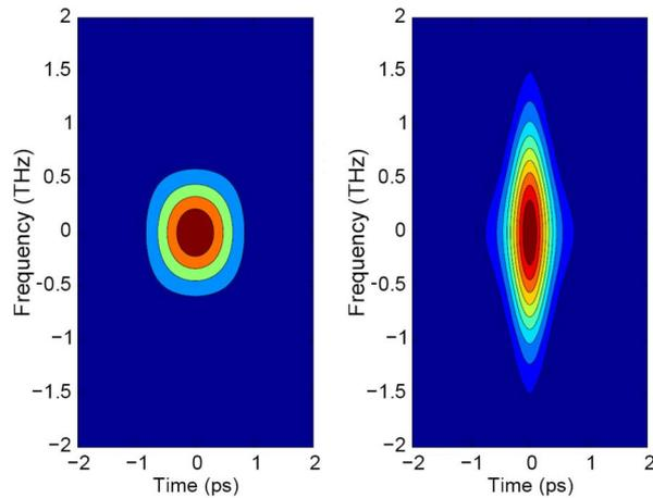
Fig. 5. Spectrogram (left) of initial pulse of 800 fs FWHM pulsedwidth with an initial peak intensity 0.33 W. Spectrogram (right) of final compressed pulse produced by self-similar process after a length of  $4L_D$ . The physical parameters are same as in Fig. 2.
