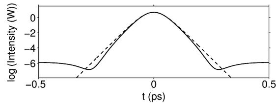
Fig. 11. Comparison of a chirped RC compressed pulse with that of hyperbolic secant pulse in logarithmic scale for the same parameter values (as in Fig. 2) for  $8L_D$  propagation distance.
