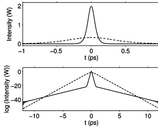
Fig. 2. Intensity profiles of initial (dashed lines) and compressed output pulse (solid lines) of a chirped solitary pulse. The physical parameters are  $\alpha_{20}/2\pi = -0.092$  GHz/ps,  $\beta_{20} = 27.24$  ps/km/nm,  $\sigma = 0.0121$ ,  $\gamma_0 = 0.1519$  W<sup>-1</sup>m<sup>-1</sup>, and  $\eta = 0.0008$ .
