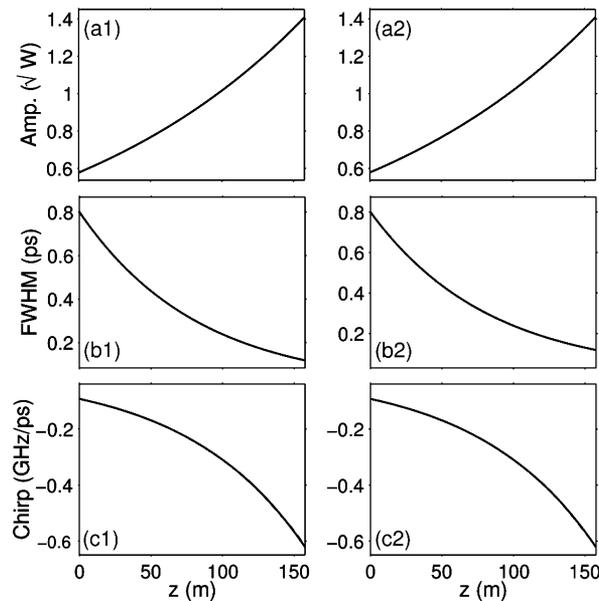
Fig. 4. Comparison of hyperbolic secant pulse evolution changes in terms of amplitude, pulsewidth, and chirp for LVM (a1, b1, c1) and CVM (a2, b2, c2). The physical parameters are same as in Fig. 2.
