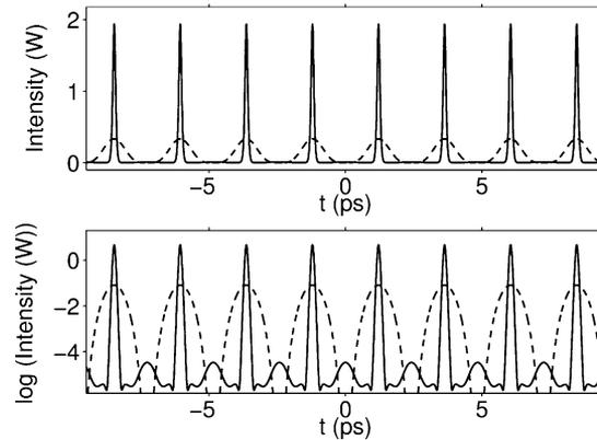
Fig. 19. Compression of a train of RC pulses in solid-core PCF over a propagation distance of  $8L_D$ . Dashed and solid lines represent the intensity plots of initial and compressed pulse trains, respectively. The parameter values are same as in Fig. 2.
