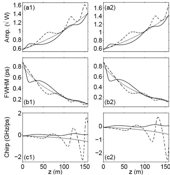
Fig. 12. Amplitude, pulsewidth, and chirp evolutions over  $8L_D$  distance propagation. In Figs. (a1), (b1), and (c1) and (a2), (b2), and (c2), the dashed lines represent the results of LVM and CVM, respectively. The solid and dotted lines correspond to full numerical and analytical results, respectively.
