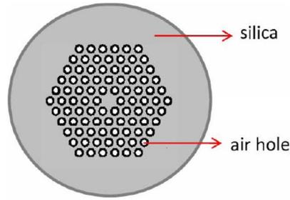
Fig. 1. Design of a tapered PCF [13].
