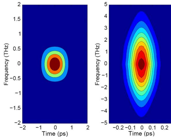
Fig. 10. Spectrogram (left) of initial RC pulse. Spectrogram (right) of final compressed pulse over a distance of  $8L_D$ . The physical parameters are same as in Fig. 2.
