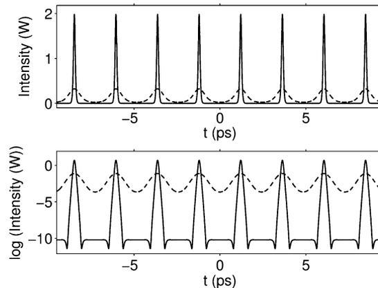
Fig. 17. Compression of a train of chirped solitary pulses in solid-core PCF over a propagation distance of  $8L_D$ . Dashed and solid lines represent the intensity plots of initial and compressed pulse trains, respectively. The parameter values are same as in Fig. 2.
