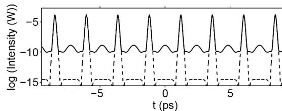
Fig. 22. Comparison of intensity plots of a train of compressed RC pulses with that of hyperbolic secant pulses in logarithmic scale in CPCF.
