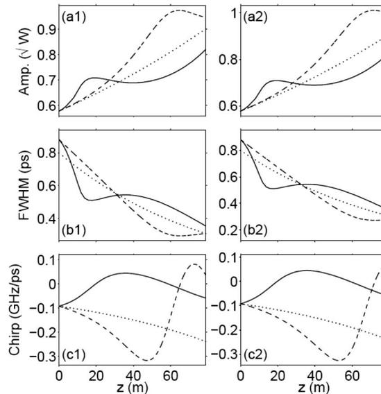
Fig. 9. Amplitude, pulsewidth, and chirp evolutions over  $4L_D$  distance propagation. In Figs. (a1), (b1), and (c1) and (a2), (b2), and (c2), the dashed lines represent the results of LVM and CVM, respectively. The solid and dotted lines correspond to full numerical and analytical results, respectively.
