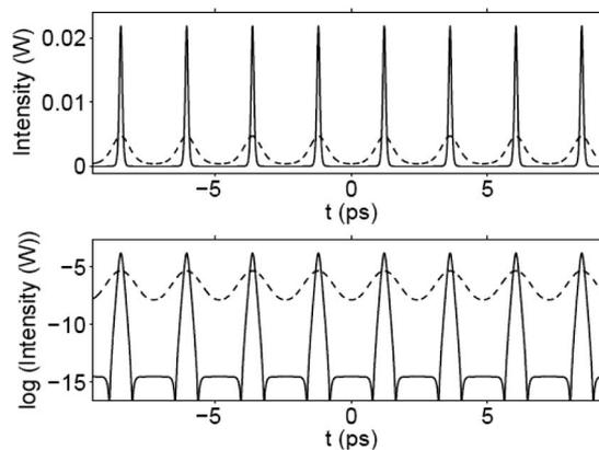
Fig. 18. Compression of a train of chirped solitary pulses in CPCF over a propagation distance of  $8L_D$ . Dashed and solid lines represent the intensity plots of initial and compressed pulse trains, respectively. The parameter values are same as in Fig. 14.
