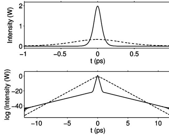
Fig. 2. Intensity profiles of initial (dashed lines) and compressed output pulse (solid lines) of a chirped solitary pulse. The physical parameters are  $\alpha_{20}/2\pi = -0.092$  GHz/ps,  $\beta_{20} = 27.24$  ps/km/nm,  $\sigma = 0.0121$ ,  $\gamma_0 = 0.1519$  W $^{-1}$ m $^{-1}$ , and  $\eta = 0.0008$ .
