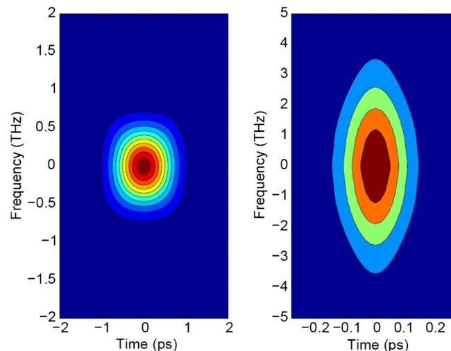
Fig. 14. Spectrogram (left) of initial RC pulse. Spectrogram (right) of final compressed pulse over a distance of  $8L_D$  in CPCF. The physical parameters are  $\alpha_{20}/2\pi = -0.092$  GHz/ps,  $\beta_{20} = 68.72$  ps/km/nm,  $\sigma = 0.03$ ,  $\gamma_0 = 26.3$  W<sup>-1</sup>m<sup>-1</sup>, and  $\eta = 0.006$ .
