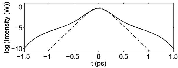
Fig. 8. Comparison of a chirped RC compressed pulse with that of hyperbolic secant pulse in logarithmic scale for the same parameter values as in Fig. 2.
