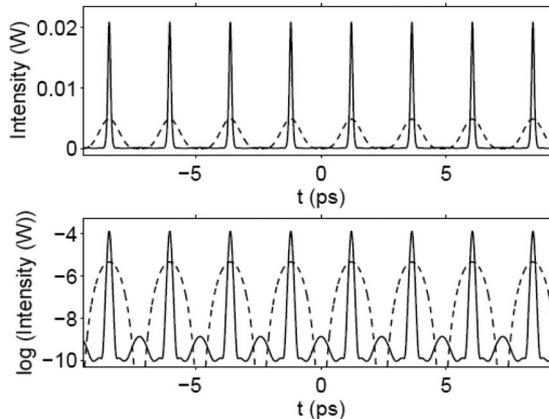
Fig. 21. Compression of a train of RC pulses in CPCF over a propagation distance of  $8L_D$ . Dashed and solid lines represent the intensity plots of initial and compressed pulse trains, respectively. The parameter values are same as in Fig. 14.
