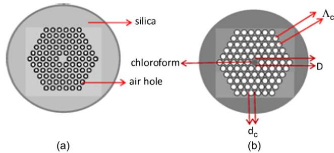
Fig. 13. (a) Schematic diagram of a solid-core PCF and a (b) CPCF [13].
