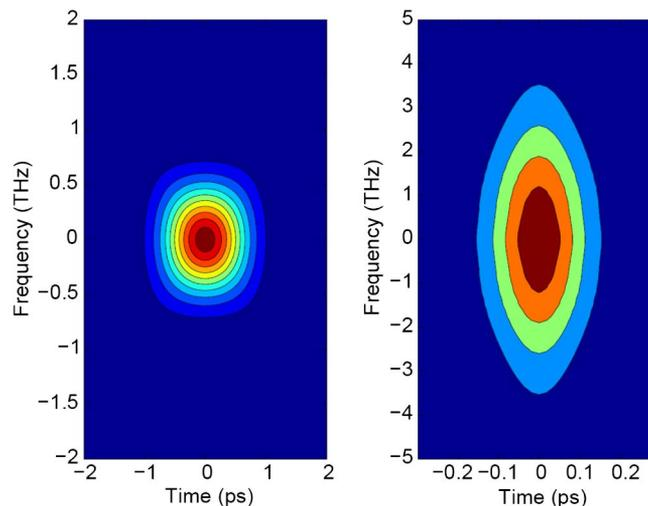
Fig. 14. Spectrogram (left) of initial RC pulse. Spectrogram (right) of final compressed pulse over a distance of  $8L_D$  in CPCF. The physical parameters are  $\alpha_{20}/2\pi = -0.092$  GHz/ps,  $\beta_{20} = 68.72$  ps/km/nm,  $\sigma = 0.03$ ,  $\gamma_0 = 26.3$  W $^{-1}$ m $^{-1}$ , and  $\eta = 0.006$ .
