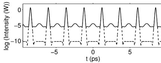
Fig. 20. Comparison of intensity plots of a train of compressed RC pulses with that of hyperbolic secant pulses in logarithmic scale.
