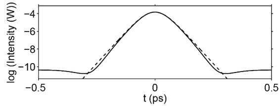
Fig. 15. Comparison of a chirped RC compressed pulse with that of hyperbolic secant pulse in logarithmic scale for the same parameter values as in Fig. 14 for  $8L_D$  in CPCF.
