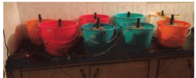
Figure 2. Accelerated corrosion test setup
