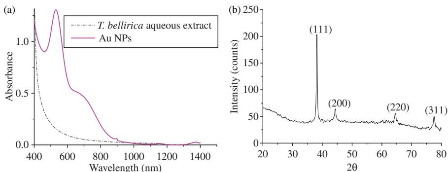
Figure 1. (a) UV-Vis spectrum of Au nanocolloids and (b) powder XRD pattern of Au NPs.
