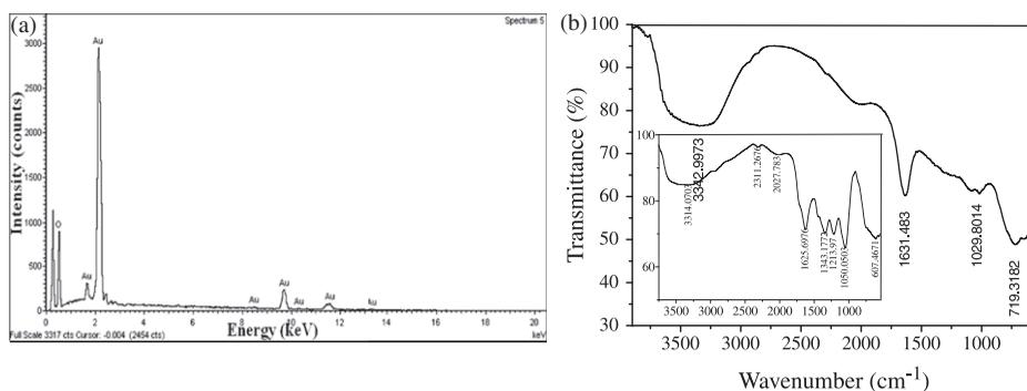
Figure 3. (a) EDAX pattern of Au NPs and (b) FT-IR spectra of Au NPs. Inset: FT-IR spectrum of *T. bellirica* dry fruit pericarp powder.
