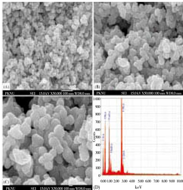
**Figure 3.** FESEM images of synthesized TiO<sub>2</sub> NPs at different resolution (A) 15 000 $\times$  (B) 30 000 $\times$  (C) 50 000 $\times$  (D) EDX showing the chemical composition.
