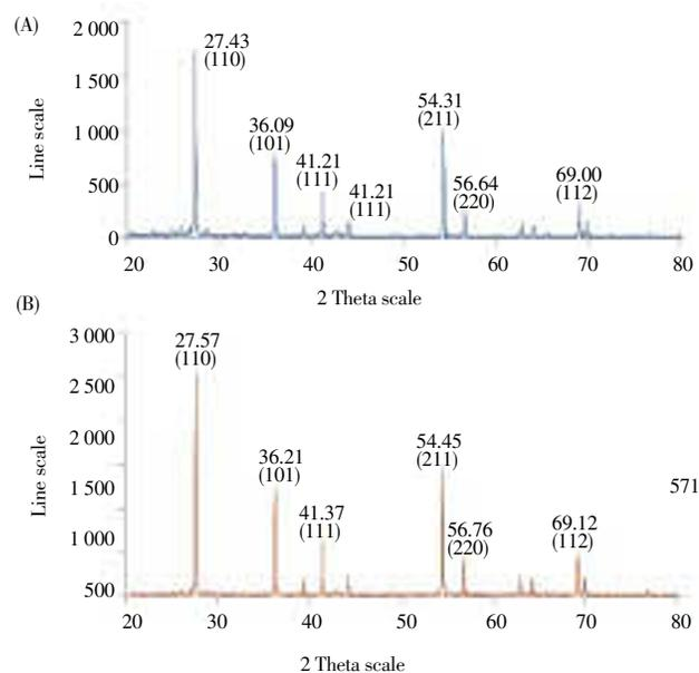
**Figure 1.** X–ray diffraction patterns of (A) Titanium dioxide, (B) Synthesized TiO<sub>2</sub> NPs.
