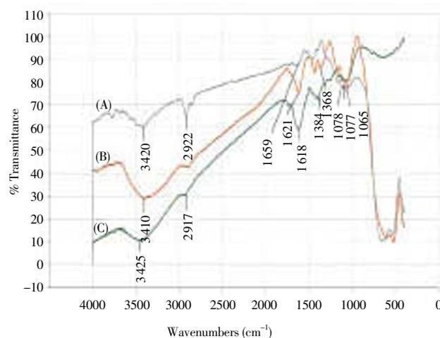
**Figure 2.** FTIR peaks of (A) Titanium dioxide, (B) Synthesized TiO<sub>2</sub> NPs, (C) *P. guajava* aqueous leaf extract.
