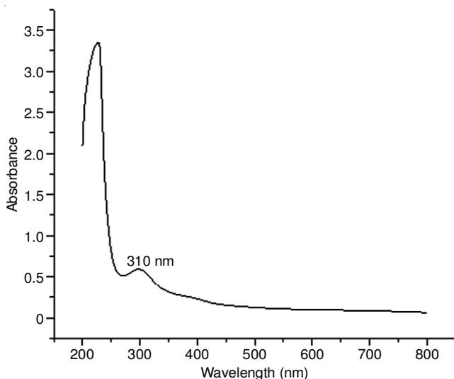
Fig. 1. UV-visible spectrum of ZnO nanoparticles
