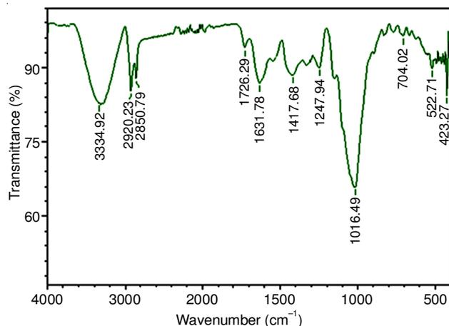
Fig. 2. FTIR spectrum of ZnO nanoparticles
