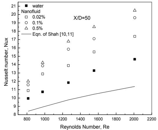
Fig 7. Variation of local Nusselt number for different volume fractions of nanofluids at X/D=50 for tube with H/D=5
