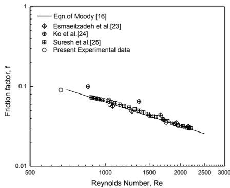
Fig 3. Comparison of friction factor for water in plain tube at different flow Reynolds number using water with data of literature
