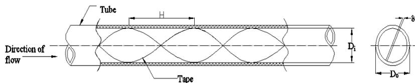
Fig. 1 (b) Full length twisted tape insert inside a tube
