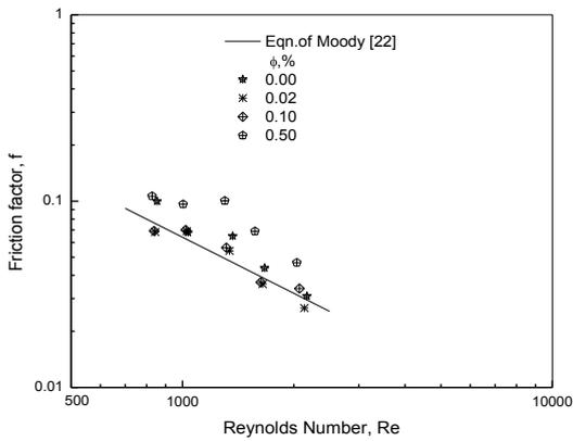
Fig 6. Variation of friction factor for water and nanofluids in plain tube at different flow Reynolds number
