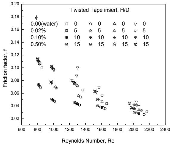
Fig 10. Variation of friction factor for different volume fractions of nanofluids and twist ratio
