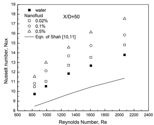
Fig 9. Variation of local Nusselt number for different volume fractions of nanofluids at X/D=50 for tube with H/D=15
