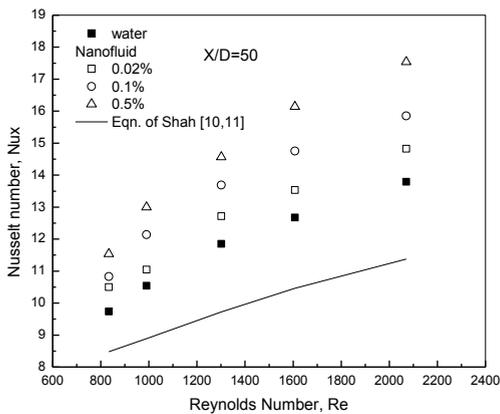
Fig 8. Variation of local Nusselt number for different volume fractions of nanofluids at X/D=50 for tube with H/D=10
