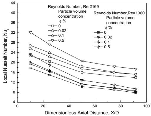
Fig 4. Variation of Local Nusselt number along the dimensionless axial distance for water in plain tube at different flow Reynolds number
