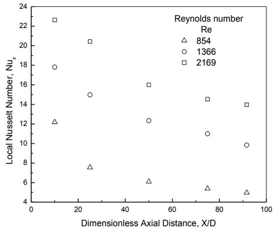
Fig 5. Variation of Local Nusselt number along the dimensionless axial distance for water and nanofluids in plain tube at different flow Reynolds number
