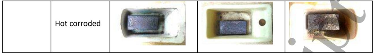
Figure 3: Macrographic images showing the air oxidized and hot corroded samples at the end of 10,20,30,40 and 50 hours
