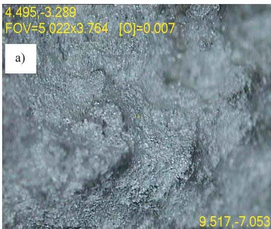
Fig. 5(a) Tensile fracture macrograph
