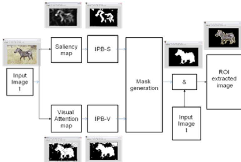
Fig 1. Step by step implementation of ROI extraction process
