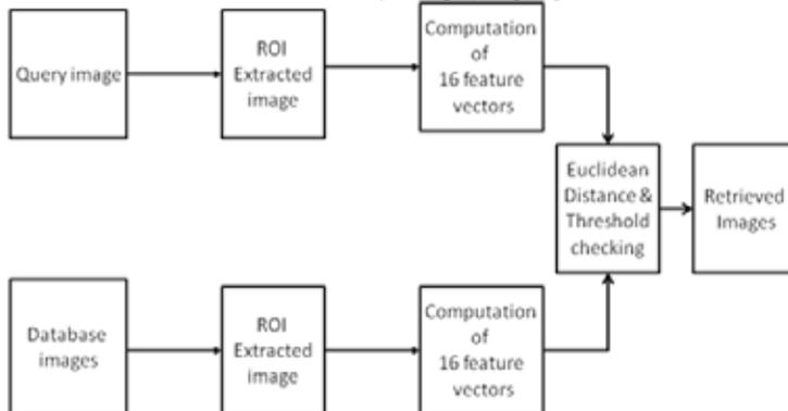
Fig 2. Block diagram of image retrieval system using ROI extraction results
