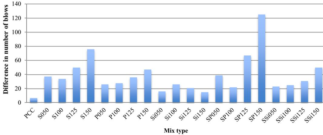
Fig. 7. Difference in number of blows after 90 days of curing.
