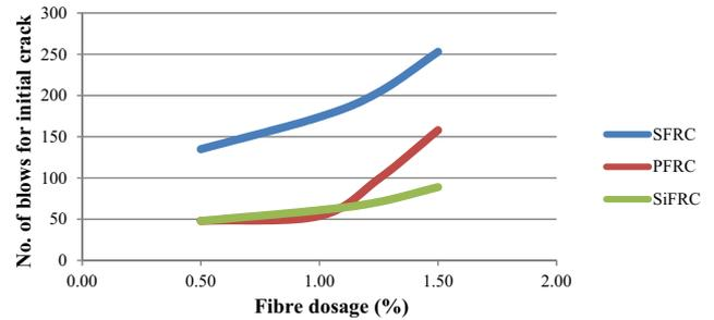
Fig. 5. Impact resistance of mono-FRC for initial crack after 90 days of curing.
