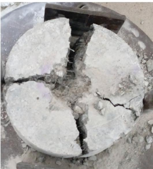
Fig. 9. Fractured specimen showing pull-out of the fibres.
