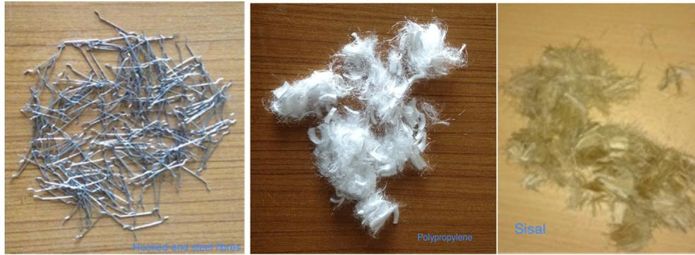
Fig. 1. Different fibres used in the experimental study.
