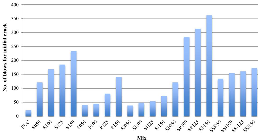
Fig. 6. Impact resistance for initial crack after 90 days of curing.
