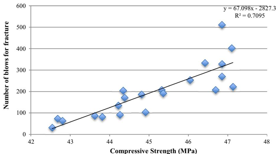
**Fig. 10.** Relation between compressive strength and no. of blows for fracture after 90 d of curing.
