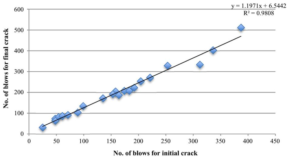
Fig. 8. Relation between number of blows for initial and final crack.
