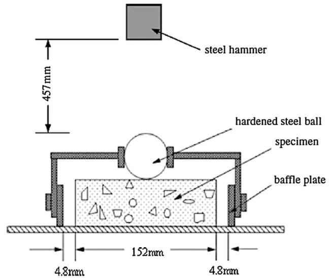
Fig. 2. Schematic diagram of drop-weight test set up.
