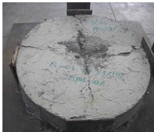
**Figure 3.** Slab specimen placed in metallic base with restrained ends.
