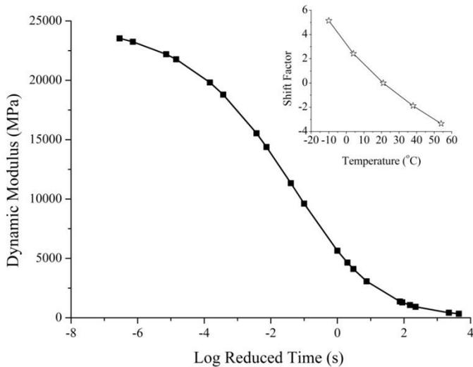
Figure 4. Master and Shift Factor for DBM Mix
