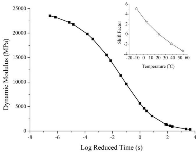
Figure 5. Master and Shift Factor for BC Mix
