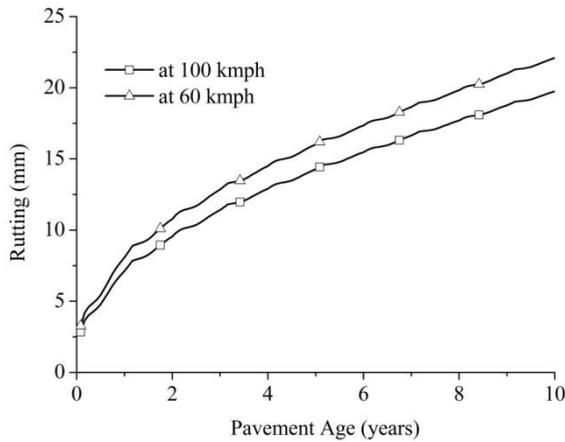
Figure 9. Comparison of Rutting at Various Traffic Speed
