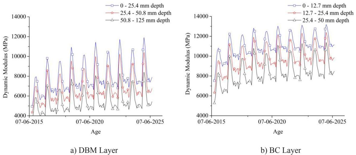
Figure 6. Dynamic Modulus at Different of BC and DBM Layer at Mid Quintile Temperature
