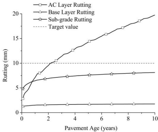
Figure 7. Rutting at different layers of the pavement
