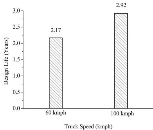
Figure 10. Design Life at Various Traffic Speed
