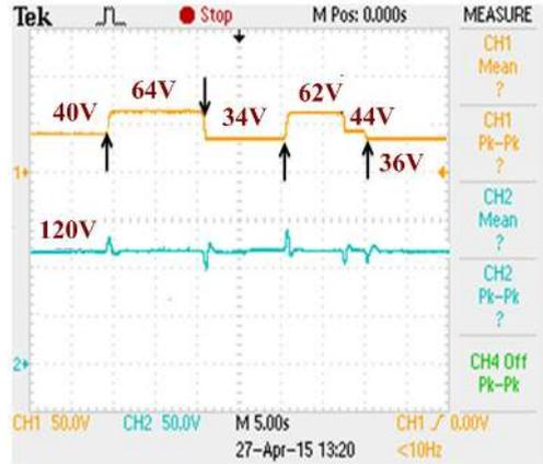
FIGURE 12. Closed-loop output waveform of FDBC in hardware.
