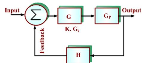
FIGURE 5. Block diagram of a closed loop plant.
