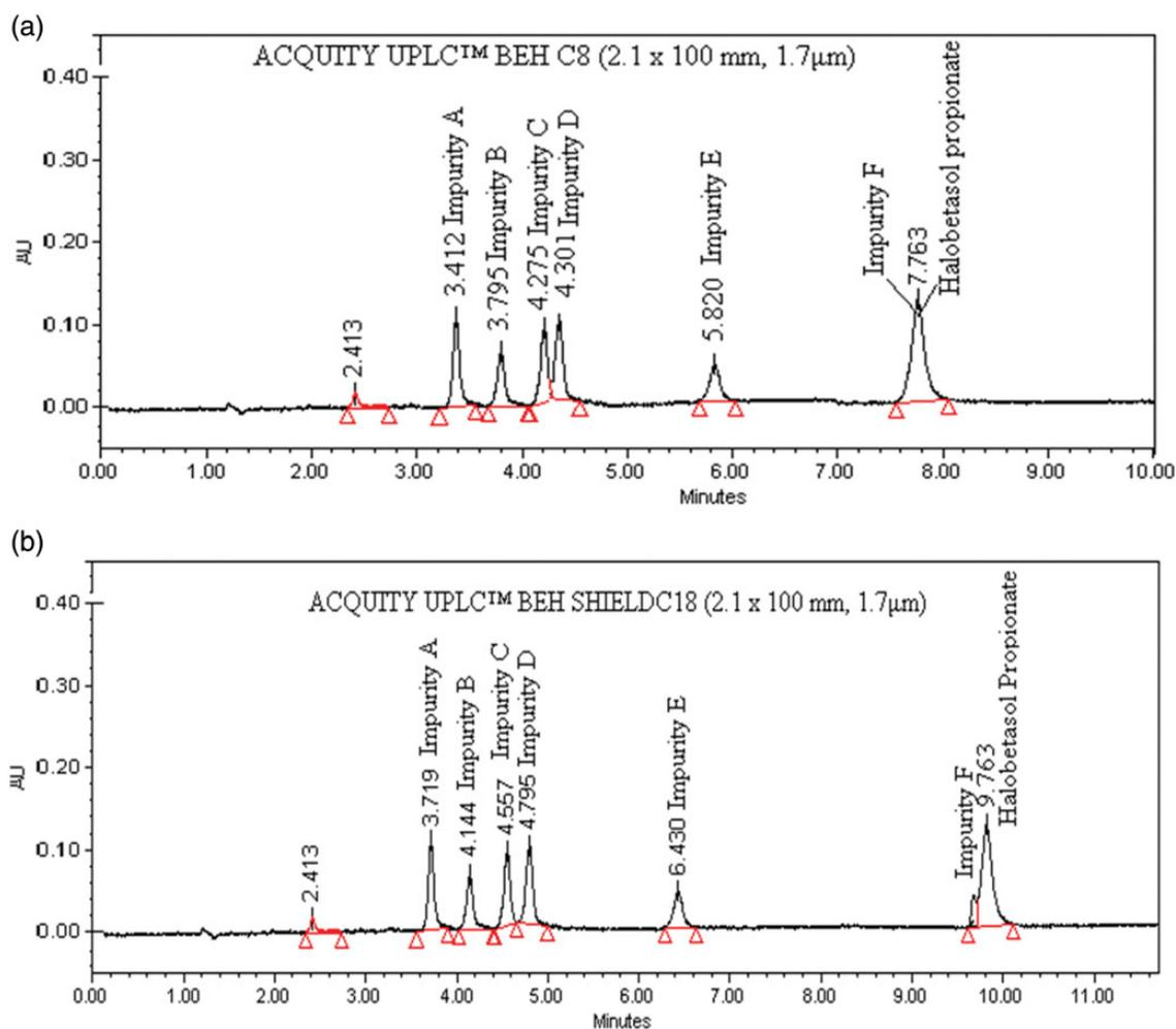
**Figure 3.** Typical chromatograms of halobetasol propionate spiked with its six impurities from method development trials: (a) typical chromatogram on ACQUITY UPLC BEH C8 (2.1 × 100 mm, 1.7 μm), (b) typical chromatogram on ACQUITY UPLC BEH SHIELD C18 (2.1 × 100 mm, 1.7 μm), (c) typical chromatogram on ACQUITY UPLC BEH Phenyl (2.1 × 100 mm, 1.7 μm)-isocratic method and (d) typical chromatogram on ACQUITY UPLC BEH Phenyl (2.1 × 100 mm, 1.7 μm)-gradient method.
