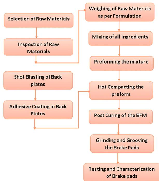
**Fig. 1.** Manufacturing process flowchart.
