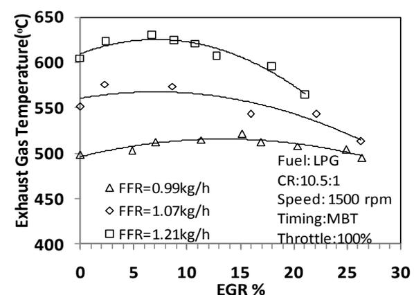
Figure 5. Variation of Exhaust Gas Temperature
