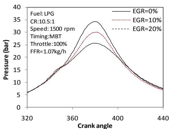
Figure 12. Variation of Pressure at FFR=1.07 kg/h
