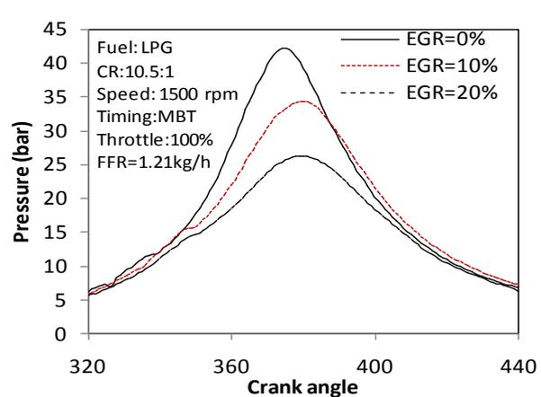
Figure 13. Variation of Pressure at FFR=1.21 kg/h
