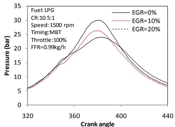
Figure 11. Variation of Pressure at FFR=0.99 kg/h
