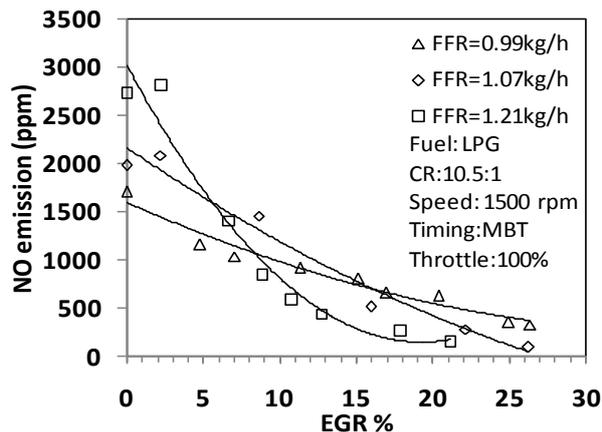
Figure 6. Variation of Nitric oxide emission
