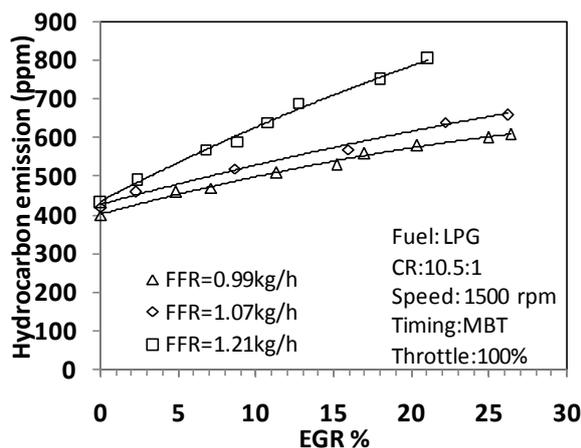
Figure 8. Variation of Hydrocarbon emission
