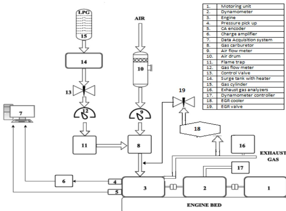
**Figure 1.** Schematic layout of Experimental Setup
