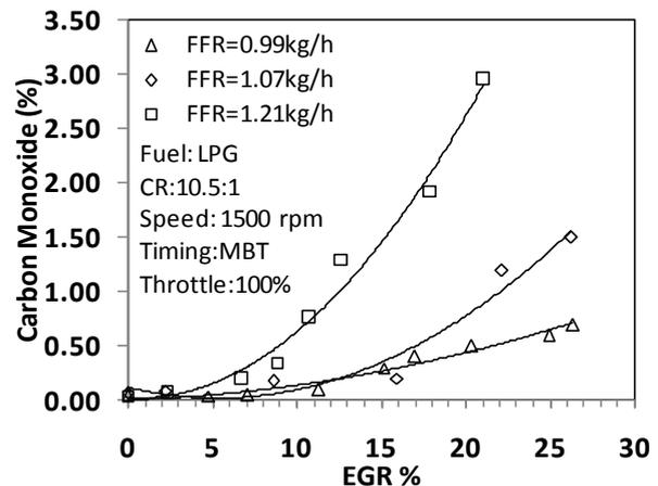
Figure 9. Variation of Carbon monoxide emission
