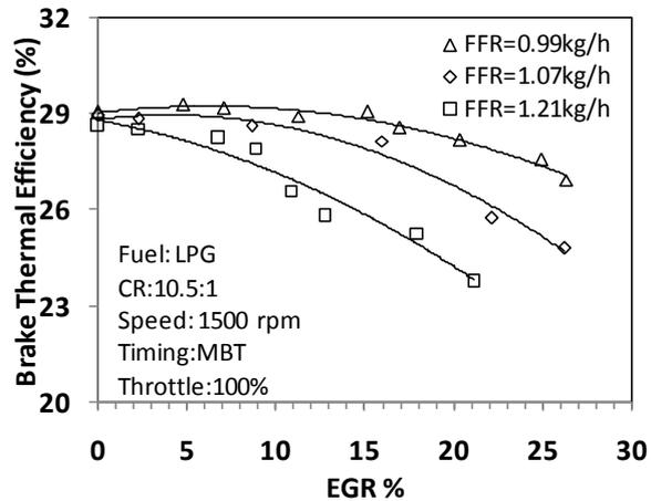
Figure 2. Variation of Brake Thermal Efficiency
