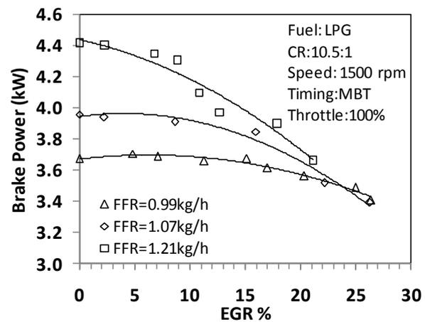
Figure 3. Variation of Brake Power with EGR
