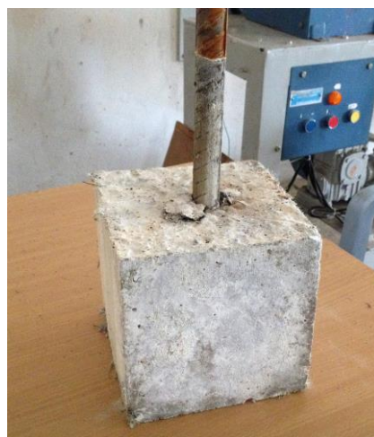
Figure 5. Test specimen after pull-out test
