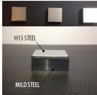
Fig.2. Photograph of Samples after coating
