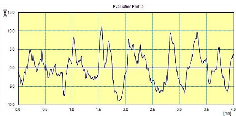
(b) Roughness profile of DSS 2205 (Ra = 3.359 μm)
