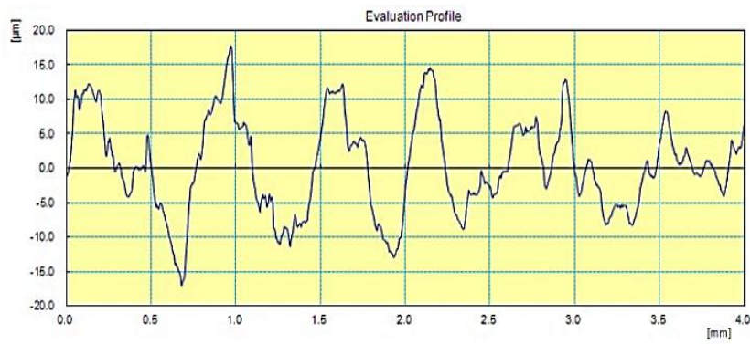
(a) Roughness profile of ASS 316L (Ra = 5.584 μm)
