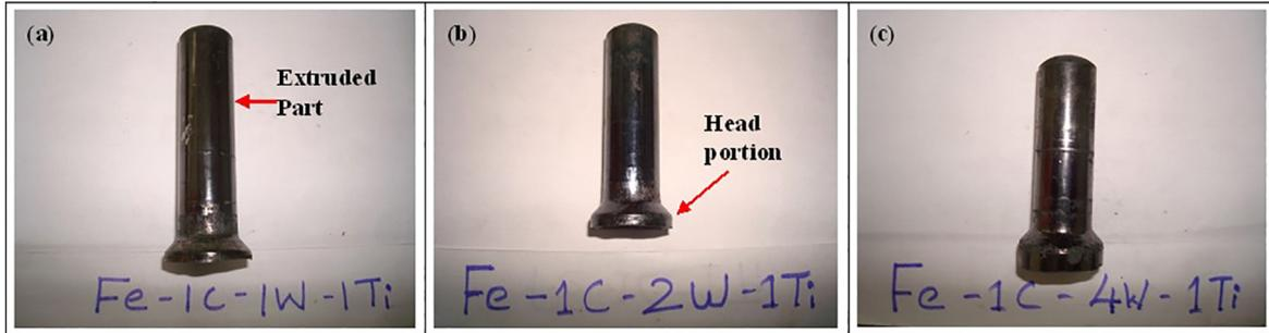
**Figure 1.** Extruded P/M alloy steels (a) Fe-1%C-1%W-1%Ti; (b) Fe-1%C-2%W-1%Ti; (c) Fe-1%C-4%W-1%Ti**Table 2.** Hardness values of P/M alloy steels for both as-sintered and hot extruded
