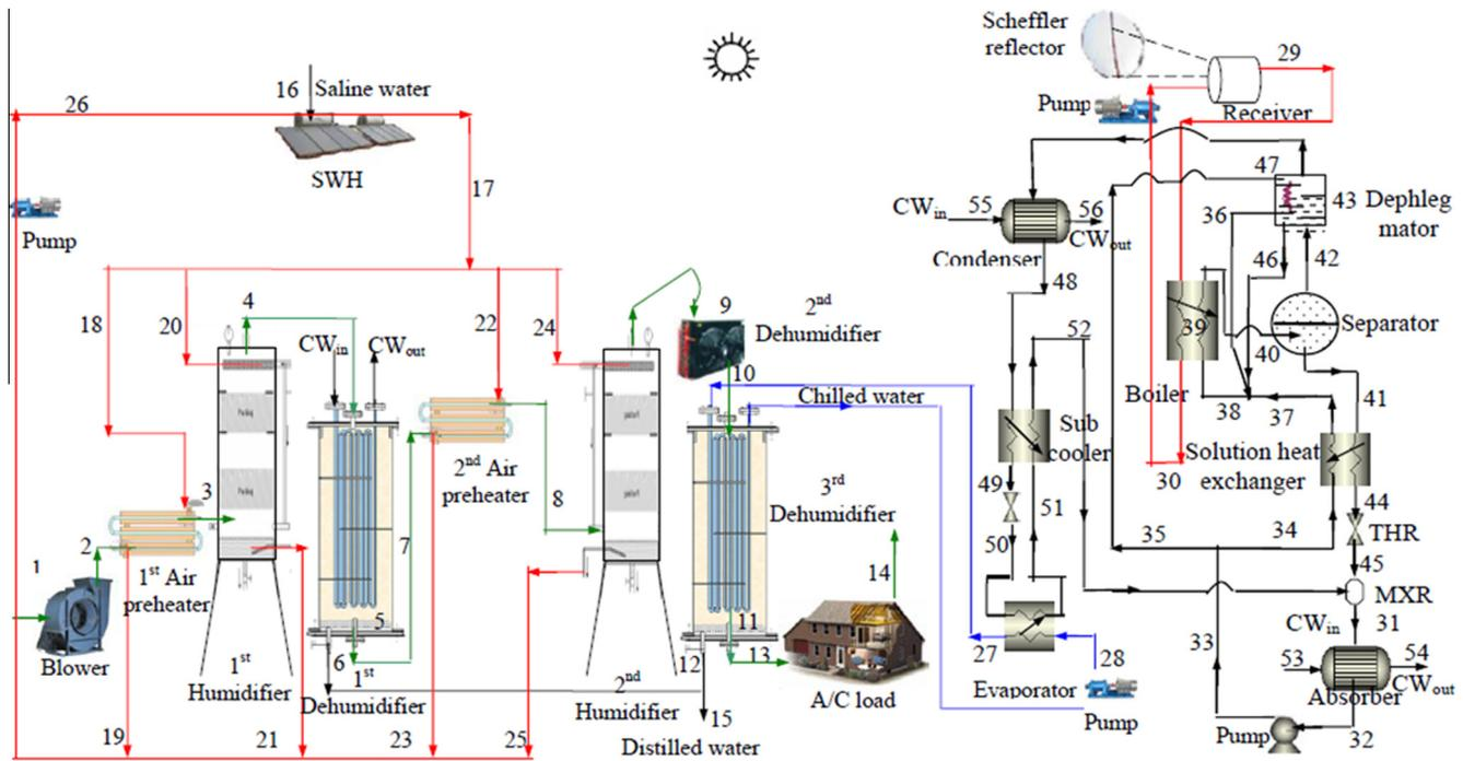
Figure 1 Two stage desalination with integrated VAR cooling.
