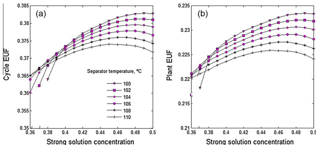
Figure 4 Influence of VAR's strong solution concentration with separator temperature on (a) cycle EUF and (b) plant EUF.
