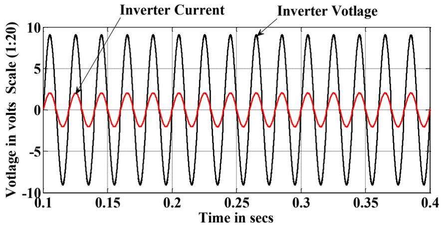
Fig. 8. Grid voltage and current for proposed system
