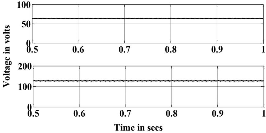
Fig. 6. Dual output boost converter output voltage waveform (upper and bottom:  $V_{e1}$  &  $V_{e2}$ )
