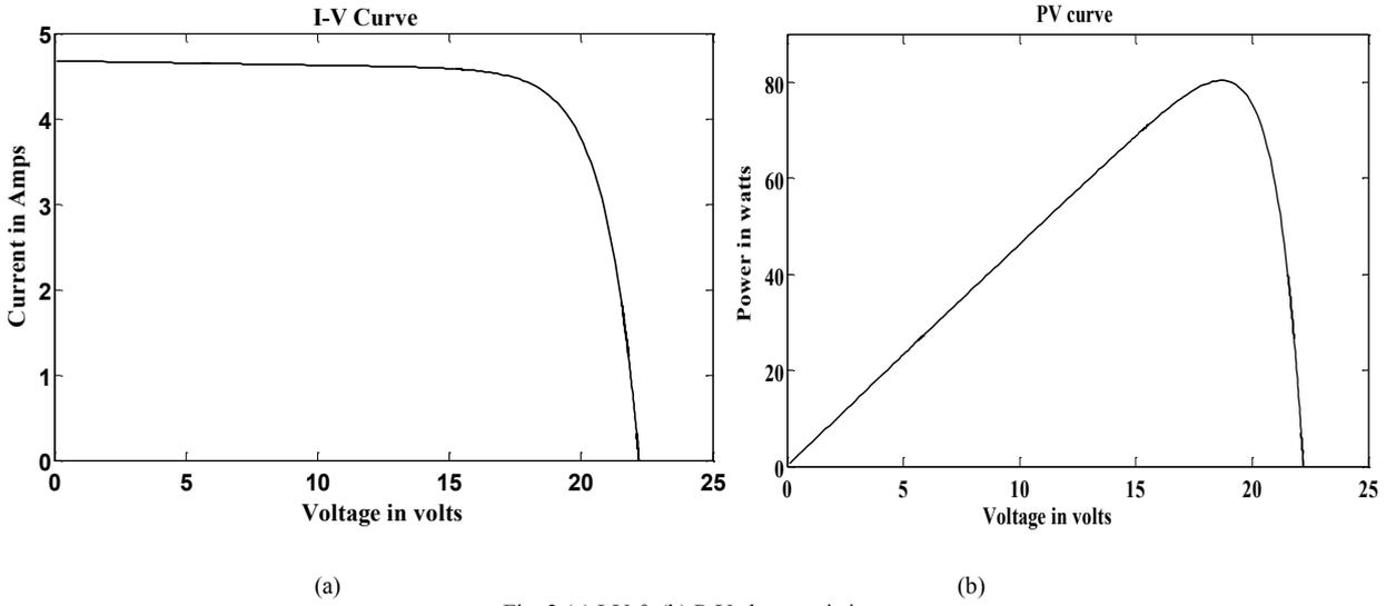
Fig. 2 (a) I-V & (b) P-V characteristics
