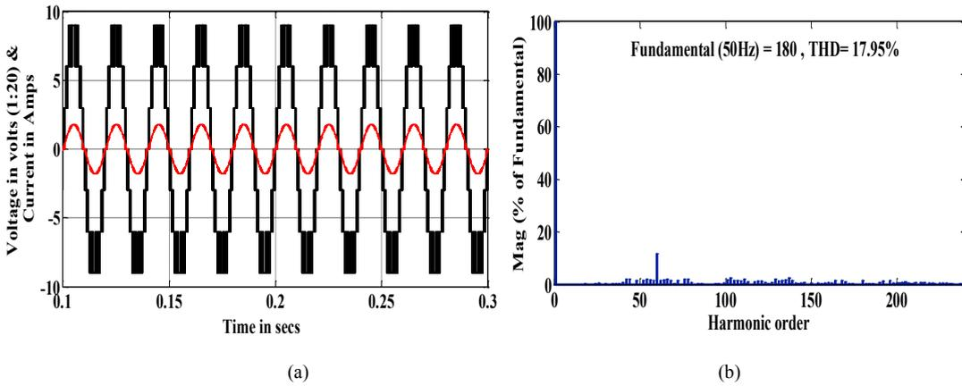
Fig. 7. (a) Output voltage and current waveform with filter (b) Harmonic spectrum plot for output voltage
