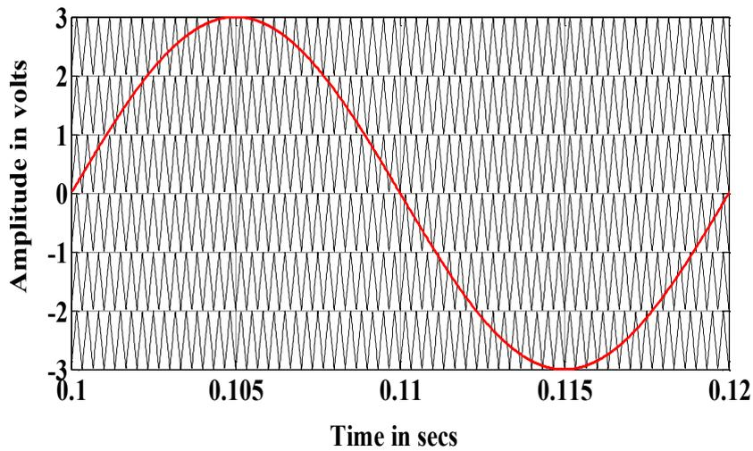
Fig. 5 Phase Disposition carrier arrangement for 7-level output voltage
