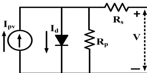
Fig. 1 Single diode model equivalent circuit
