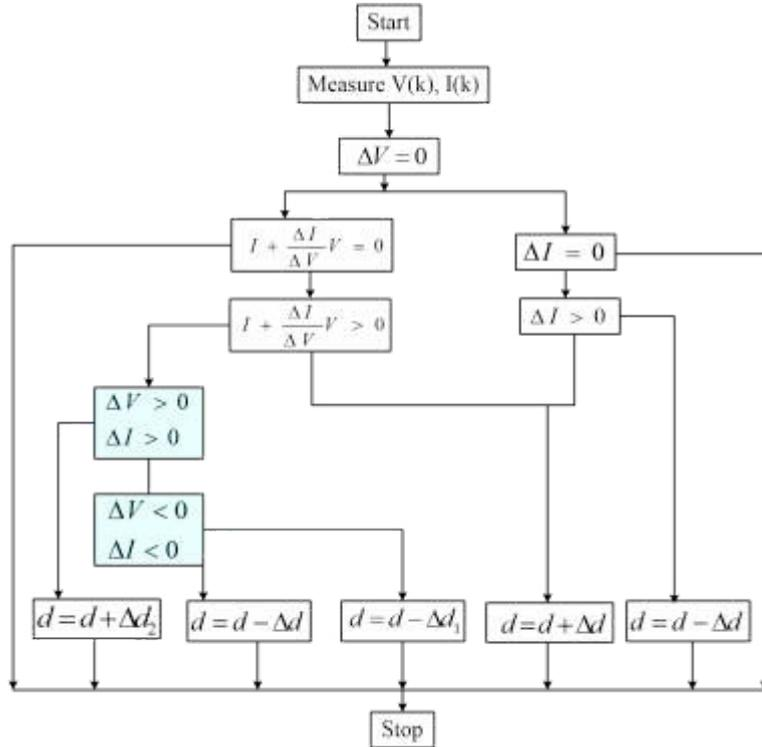
Fig. 3 Improved Incremental and Conductance MPPT algorithm
