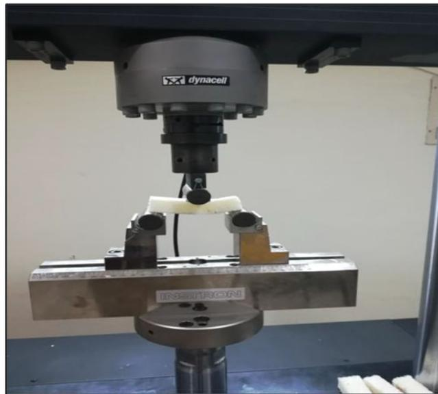
Figure 3. Flexural test specimen.
