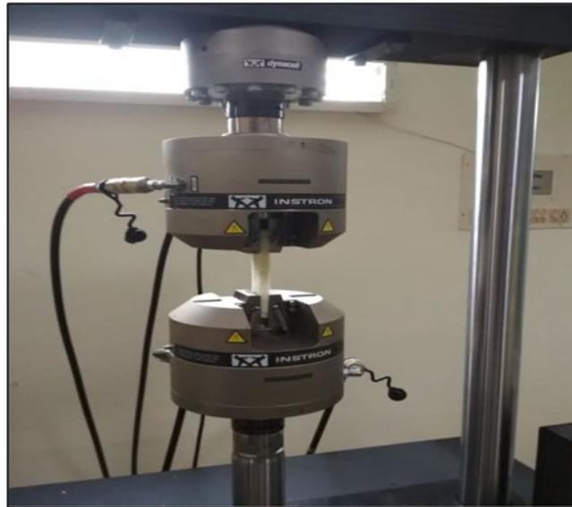
Figure 2. Tensile test specimen.
