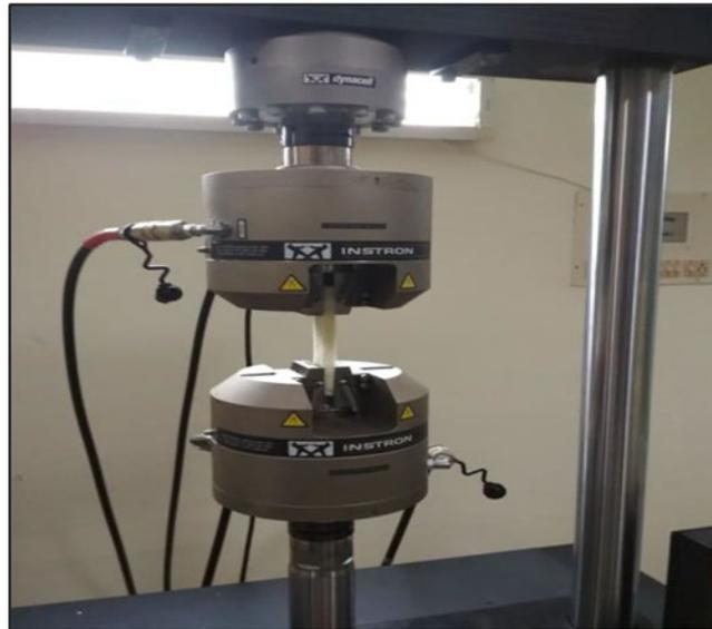
Figure 2. Tensile test specimen.
