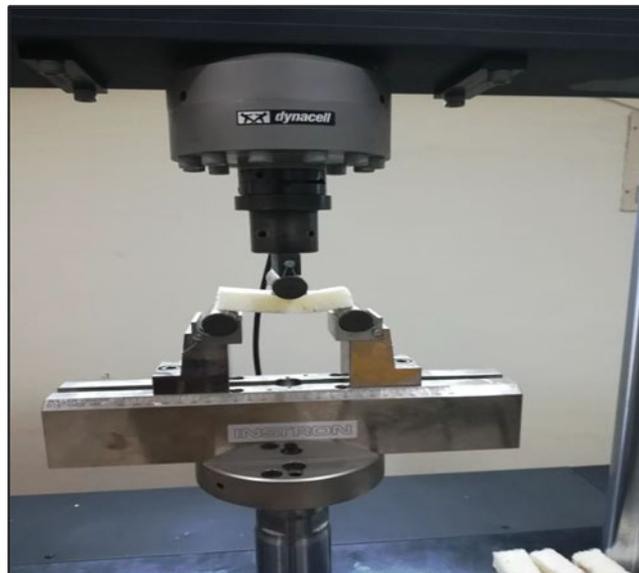
Figure 3. Flexural test specimen.
