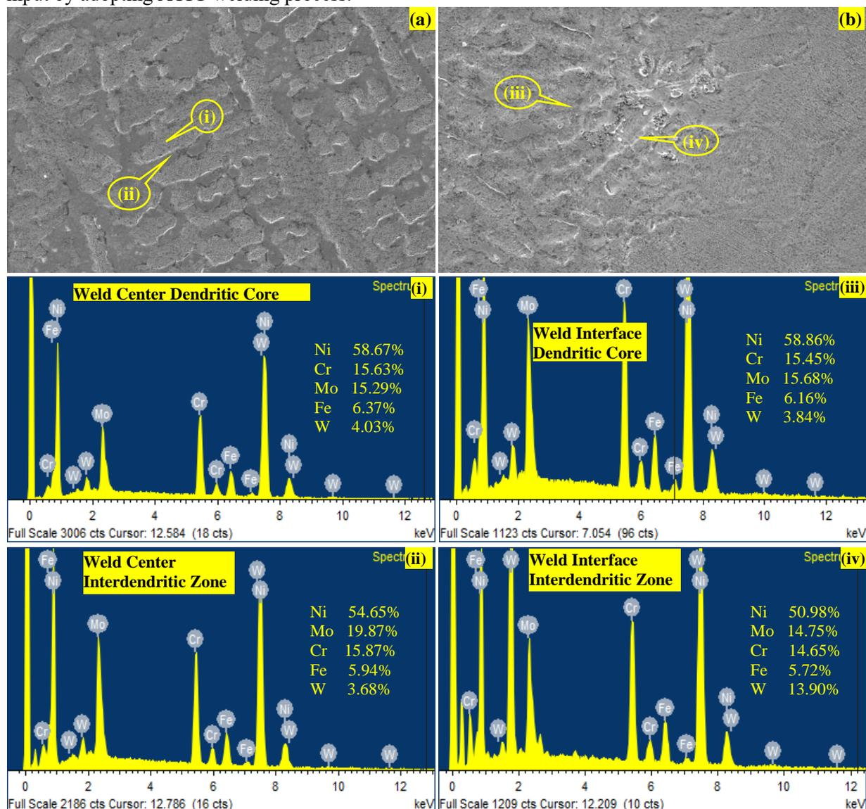
Figure 4 SEM/EDAX analysis of ATIG welded C-276 alloy for different places of weldment a) SEM-Weld Center; b) SEM-Weld Interface; i)Weld Center- Dendritic Core; ii) Weld Center- Interdendritic Zone; iii)Weld Interface- Dendritic Core; iv) Weld Interface- Interdendritic Zone
