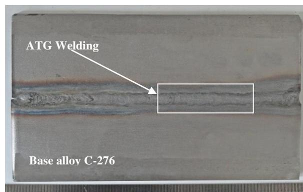
Figure 1 Photograph of Alloy C-276 ATIG Weldment
