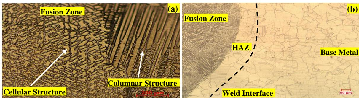
Figure 3 Microstructure of ATIG welded alloy C-276 alloy a) Fusion Zone; b) Weld Interface
