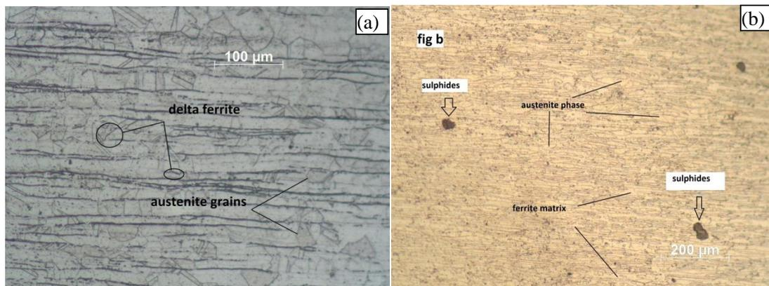
**Figure 2.** Base metal microstructure (a) AISI 316L and (b) Duplex 2205
