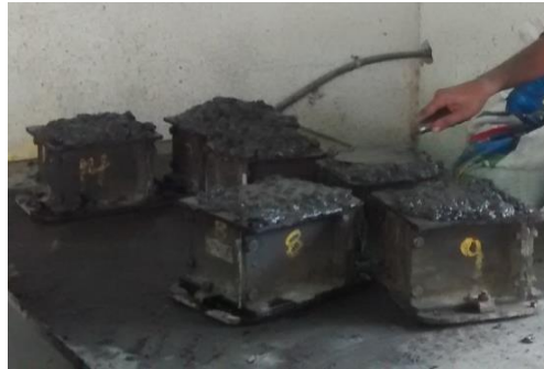
Figure 1: Casting of TBC specimens
