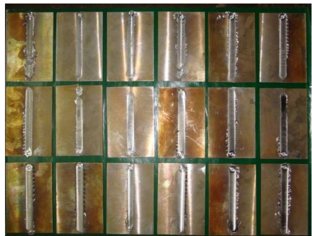
Figure 4. Photographs of the part of the joint specimens fabricated by FSW using the three different tool profiles at various tool rotational speeds
