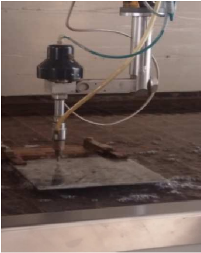
Figure 2. Water jet cutting process of the specimen
