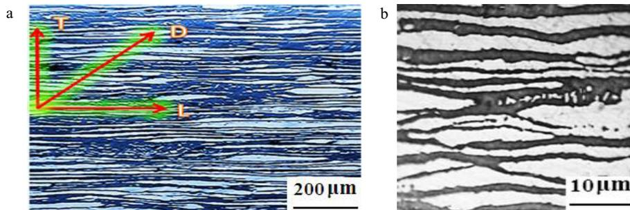
Fig.2 (a) DSS parent metal microstructure (b) Elongation of grains in the rolling direction
