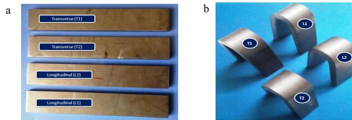
Fig.7. Bend test samples (a) Before bending (b) After bending
