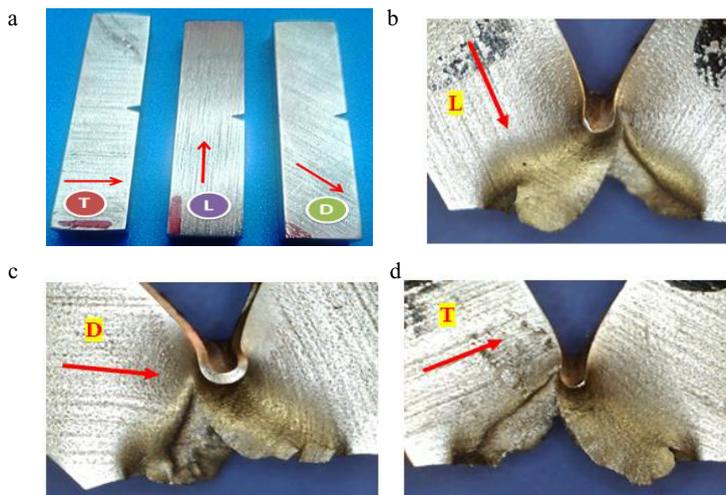
Fig.4. Plastic deformation (a) Notches in different directions (b) Longitudinal sample (c) Diagonal samples (d) Transverse sample
