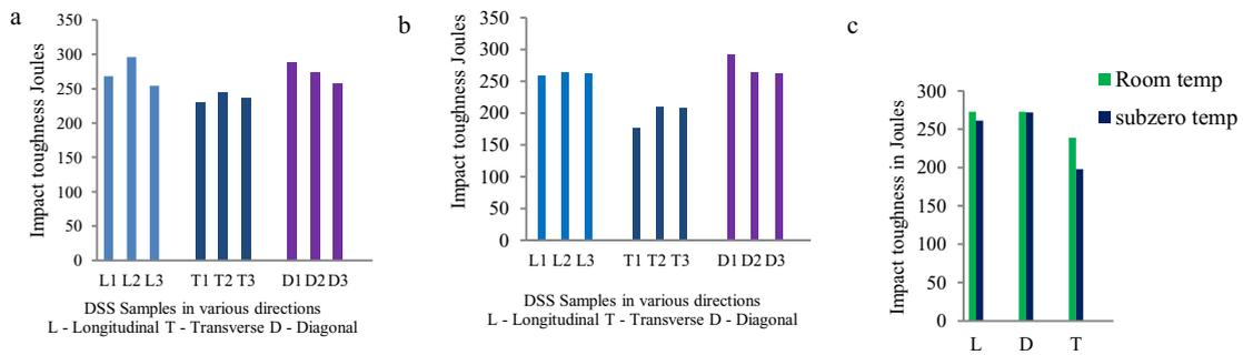
Fig.3. Impact toughness (a) At room temperature (b) At subzero temperature (c) Comparison of average impact toughness
