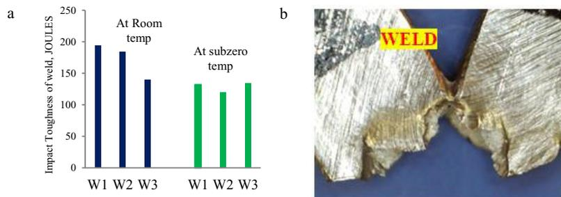
Fig.9. (a) Impact toughness of DSS weld (b) Cleavage fractured of DSS weld sample
