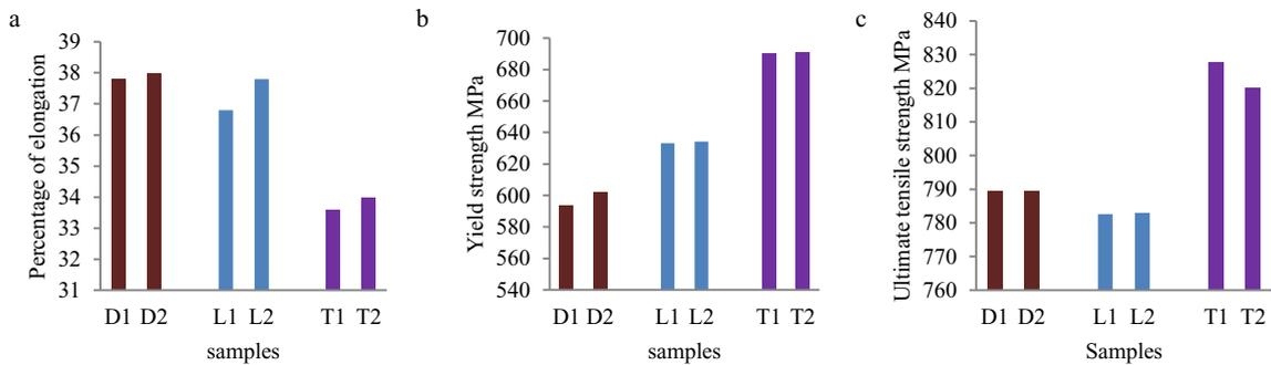
Fig.5. Tensile properties of DSS (a) Percentage of elongation (b) Yield strength (c) Ultimate tensile strength
