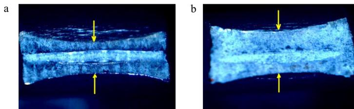
Fig.6. Fractured surface (a) Longitudinal direction (b) Transverse direction
