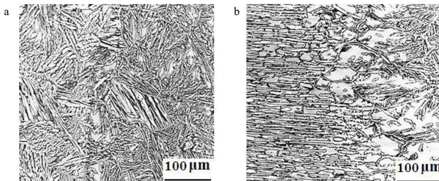
Fig.8. DSS Weld microstructure (a) Weld (b) HTHAZ
