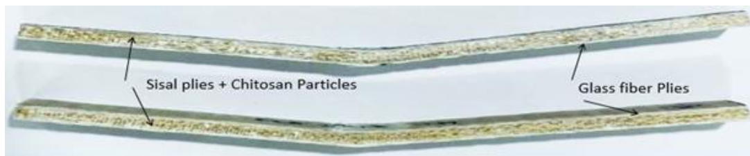
Figure 6. GF/SF/CTS hybrid sandwich composite scaffolds in a three-point bending.
