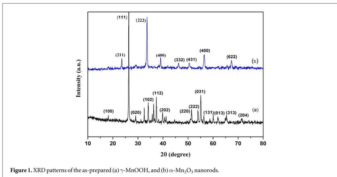
Figure 1. XRD patterns of the as-prepared (a)  $\gamma$ -MnOOH, and (b)  $\alpha$ -Mn<sub>2</sub>O<sub>3</sub> nanorods.
