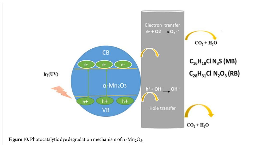
**Figure 10.** Photocatalytic dye degradation mechanism of  $\alpha$ - $\text{Mn}_2\text{O}_3$ .
