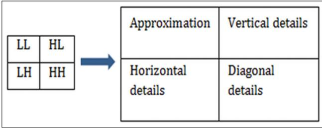
Fig. 3: Discrete wavelet transform subband decomposition
