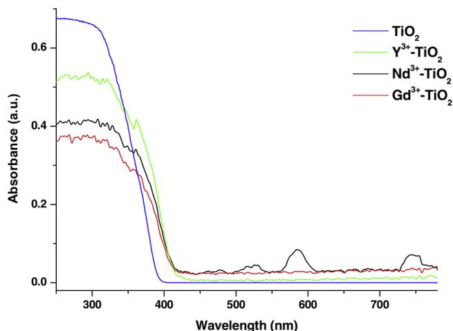
Fig. 5. Diffuse reflectance UV-Vis (DR-UV-Vis) analysis of bare and RE loaded TiO<sub>2</sub> nanocatalysts.
