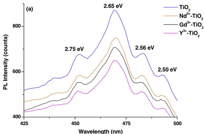
Fig. 4. Emission spectrum of the various nanocatalysts excited at 275 nm.
