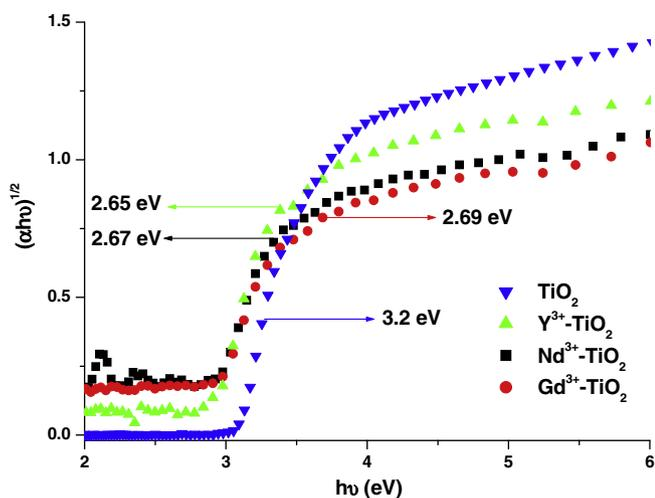
Fig. 6. The Tauc plot derived from the Kubelka Munk function for the various nanocatalysts using DR UV-Vis spectrum.
