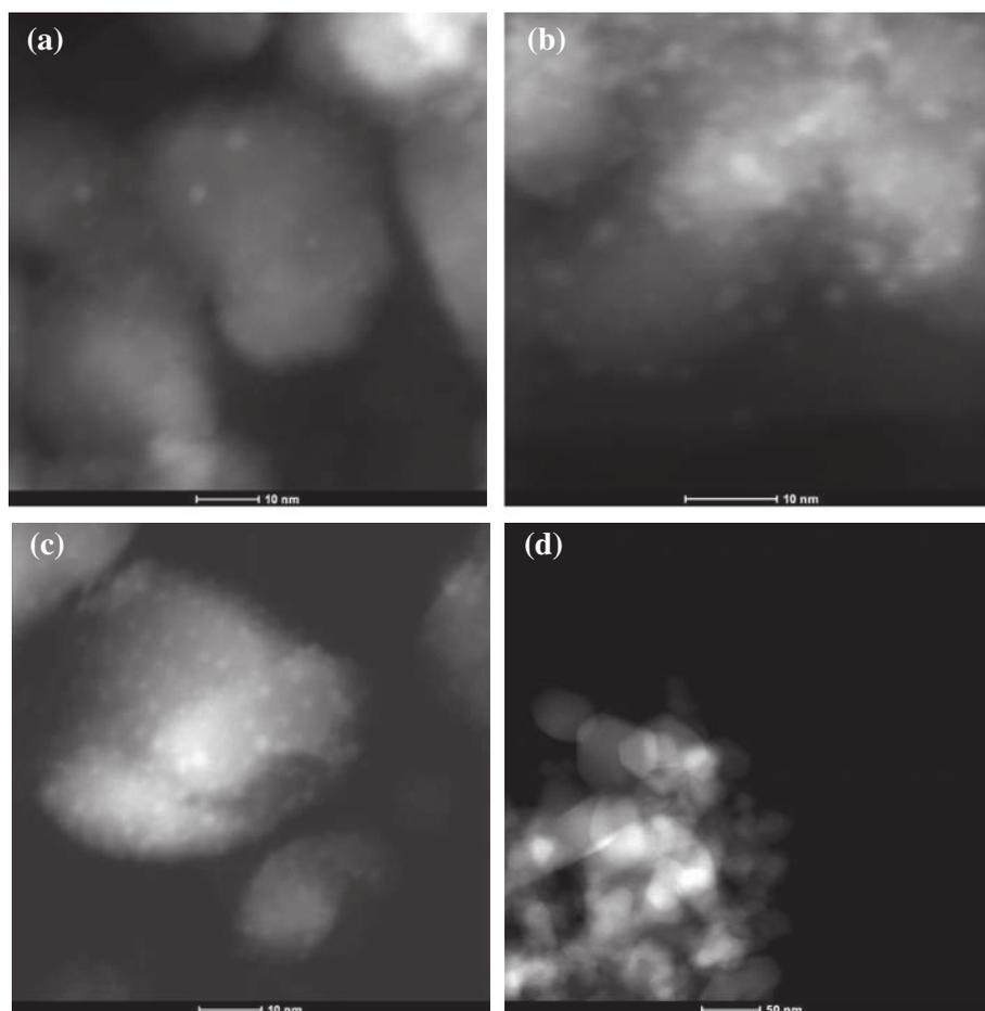
Fig. 2. STEM-HAADF images of (a)  $\text{Gd}^{3+}$ , (b)  $\text{Nd}^{3+}$  and (c)  $\text{Y}^{3+}$  loaded  $\text{TiO}_2$  nanocatalysts and (d) corresponds to the bare  $\text{TiO}_2$ .
