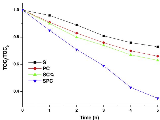
Fig. 7. Total organic carbon (TOC) removal of AB113 during various advanced oxidation processes ((S) sonolysis, (PC) photocatalysis, (SC) sonocatalysis and (SPC) sonophotocatalysis) in the presence and absence of  $Y^{3+}$  loaded  $TiO_2$ .
