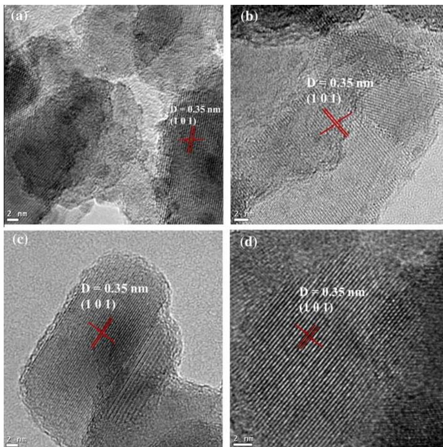
Fig. 3. HRTEM micrographs of (a)  $\text{Gd}^{3+}$ , (b)  $\text{Nd}^{3+}$  and (c)  $\text{Y}^{3+}$  loaded  $\text{TiO}_2$  nanocatalysts and (d) corresponds to the bare  $\text{TiO}_2$ .
