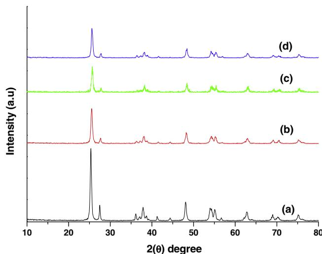
Fig. 1. X-ray diffraction pattern of bare (a) and RE ((b) Gd<sup>3+</sup>, (c) Nd<sup>3+</sup> and (d) Y<sup>3+</sup> loaded TiO<sub>2</sub> nanocatalysts.
