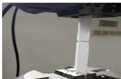
Figure 4. Tensile failure point
