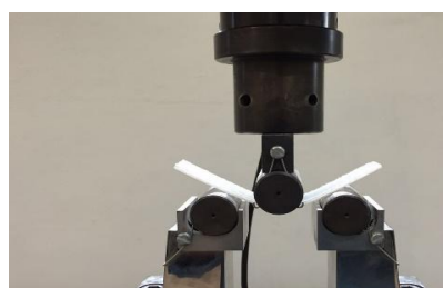
Figure 5. Flexural failure point
