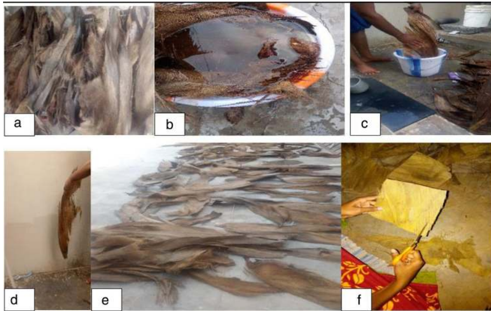
Fig. 3 – Extraction of Cocos nucifera sheath (a) waste Cocos nucifera sheath, (b) dipped sheath, (c) tap water cleaning, (d) distilled water cleaning, (e) drying process, and (f) cutting the sheath to the required size.
