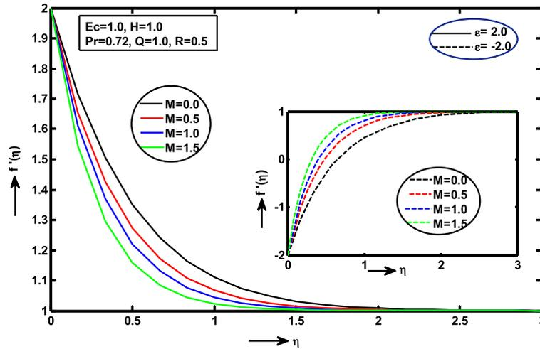
Fig. 4. Velocity profiles for various values of  $M$ .
